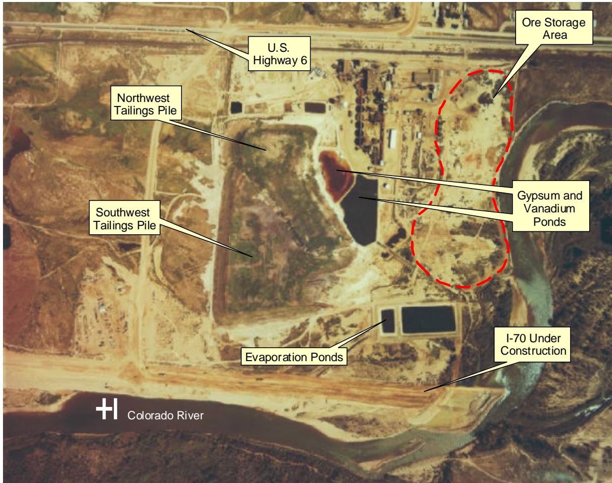
Figure 2. August 1974 View of the New Rifle Millsite, Showing the Northwest and Southwest Tailings Piles, Holding Ponds, Mill Buildings, and Ore Storage Area
