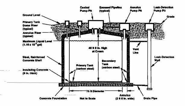
Figure 1. Single-Shell and Double-Shell Tank Configurations.
