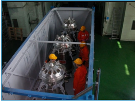
NNSA workers load casks of highly enriched uranium nuclear fuel for shipment out of Romania.
