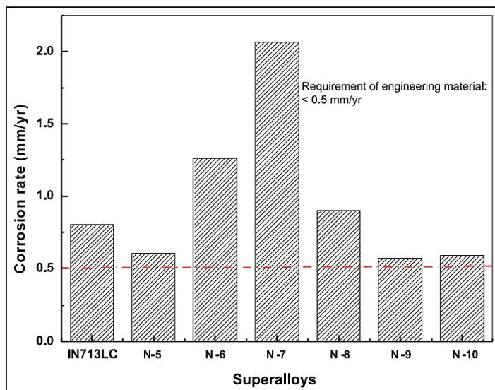
Figure 1. Corrosion rate of Alloys N5 through N10.
