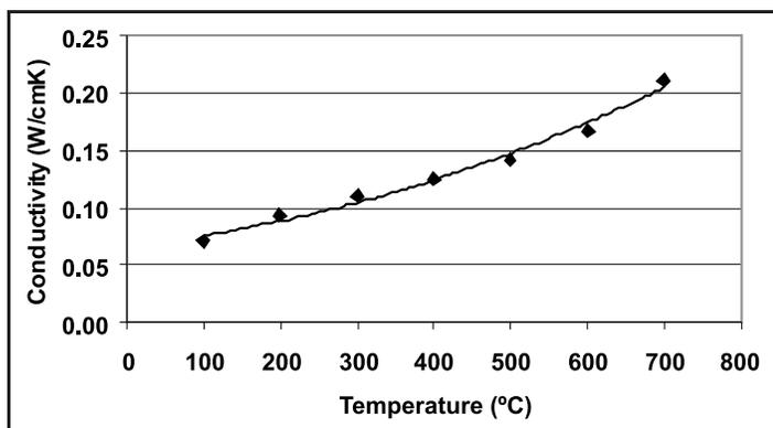
Figure 4. Plot of thermal conductivity values from correlated fitted data for an AFC-2 irradiation test fuel alloy sample.
