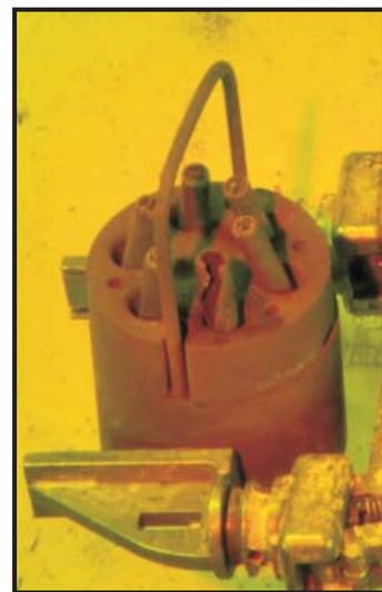
Figure 1. Photograph of MOX fuel following advanced voloxidation testing.
