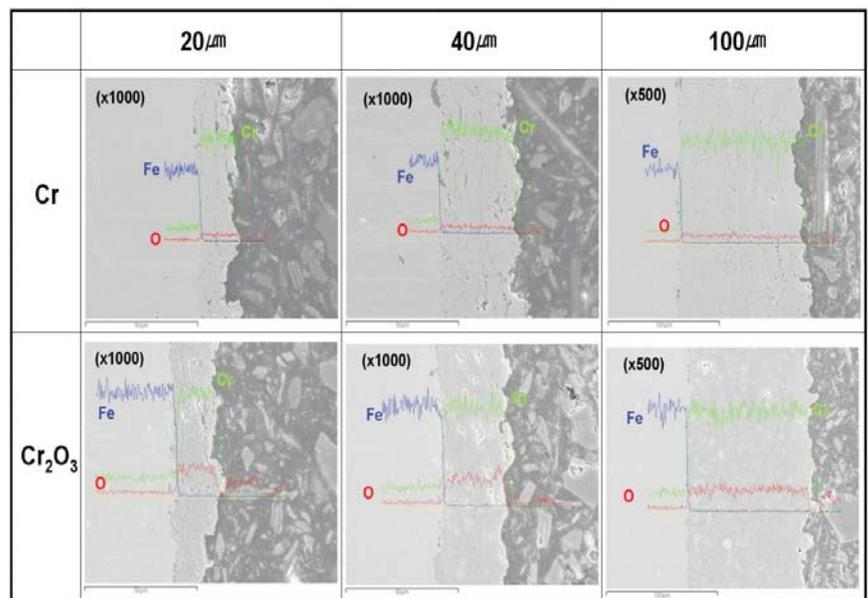
Figure 2. Microstructures of Cr and  $\text{Cr}_2\text{O}_3$  plasma spray coating.
