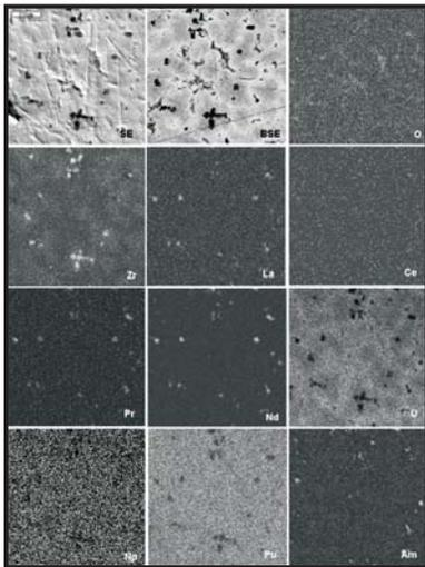
Figure 2. SE, BSE, and WDS x-ray maps from the interior of an AFC-2 irradiation test series fuel sample.
