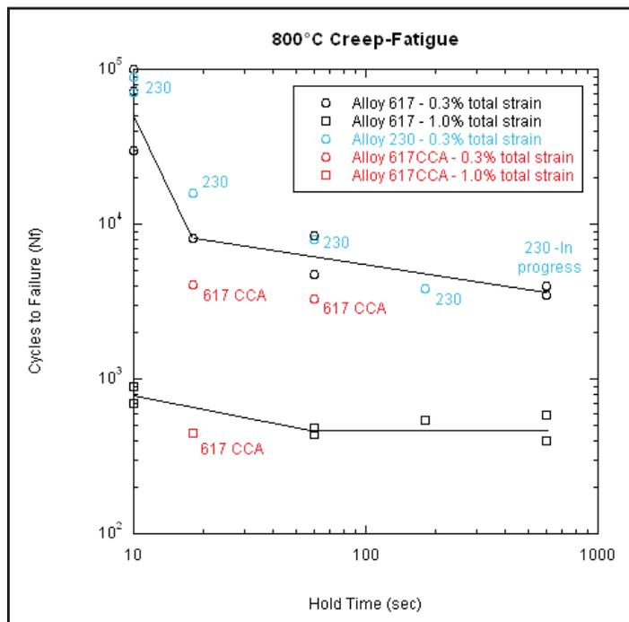
Figure 3. Cycles to failure in creep fatigue as a function of the tensile hold time. The black symbols represent tests carried out in the NGNP R&D program on 20 mm-thick plate material from a commercial vendor. The colored symbols (labeled with the alloy number designation) represent recent results for Haynes 230 and for a CCA version of Inconel 617.
