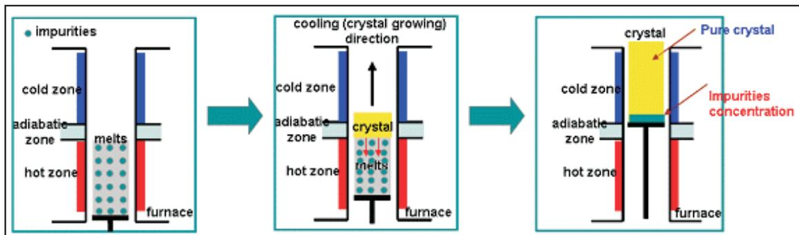
Figure 2. Zone-freezing process for fission product separation/electrorefiner salt purification.
