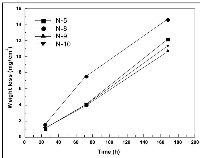
Figure 2. Weight loss of cast Ni-base alloys corroded at 650°C as a function of time.
