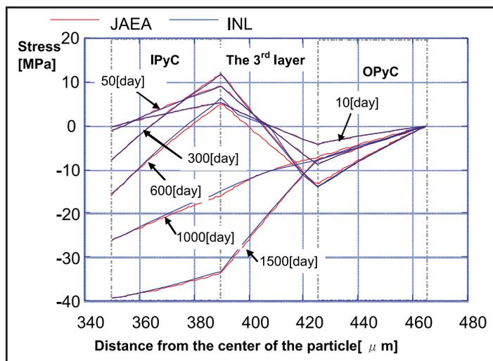
Figure 2. Radial stress distribution in TRISO fuel coating system calculated by fuel performance codes developed by JAEA and INL.
