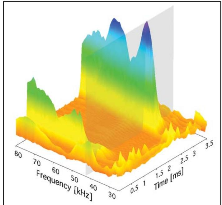
Figure 1. Ultrasonic reflection signal for prototype level measurement system.
