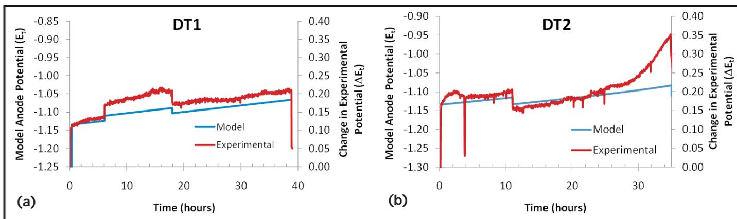
Figure 1. Anode potential comparison for two runs in repeatability tests.
