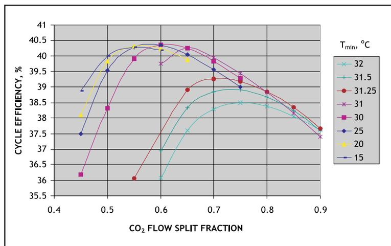
Figure 3. S-CO<sub>2</sub> Brayton cycle efficiency versus temperature and flow split between main and recompressing compressors for minimum pressure of 7.4 MPa.
