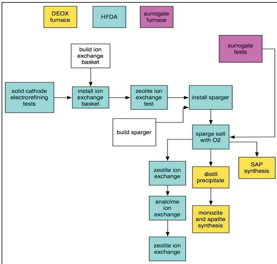
Figure 3. Proposed experimental plan for fission product removal from actual electrorefiner salt.
