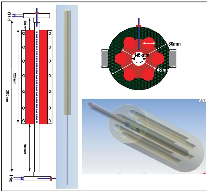
Figure 2. Circular channel test section for measurement of heat transfer coefficients for supercritical CO<sub>2</sub>.
