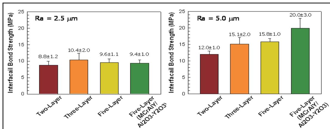
Figure 3. Interfacial bond strength of functional gradient YSZ coatings.
