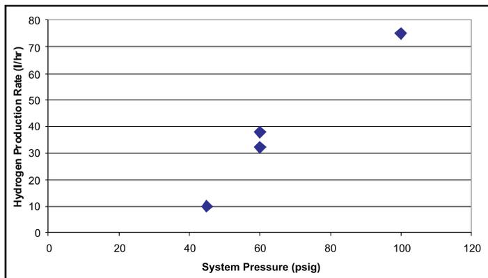
Figure 2. H<sub>2</sub> production rate as a function of pressure in the HI decomposition section.
