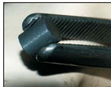
Figure 1. AFC-2 C/D fuel pellet containing 2 wt% Np and 3 wt% Am.
