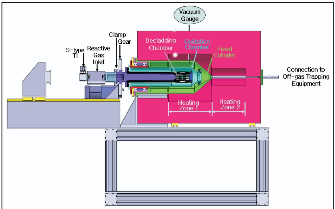
Figure 2. Schematic of advanced rotary-type voloxidizer designed by KAERI.
