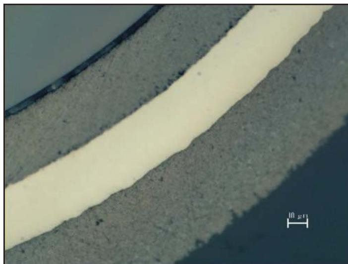
Figure 1. Cross-sectional micrograph of ZrC and pyrocarbon layers produced in a continuous deposition process.
