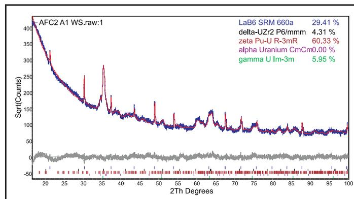
Figure 1. Rietveld refinement analysis results from an AFC-2 irradiation test series alloy.
