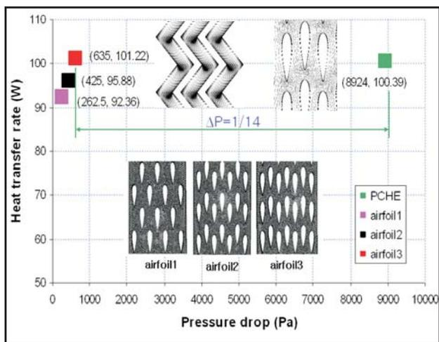
Figure 2. Calculated pressure drop for different channel configurations.
