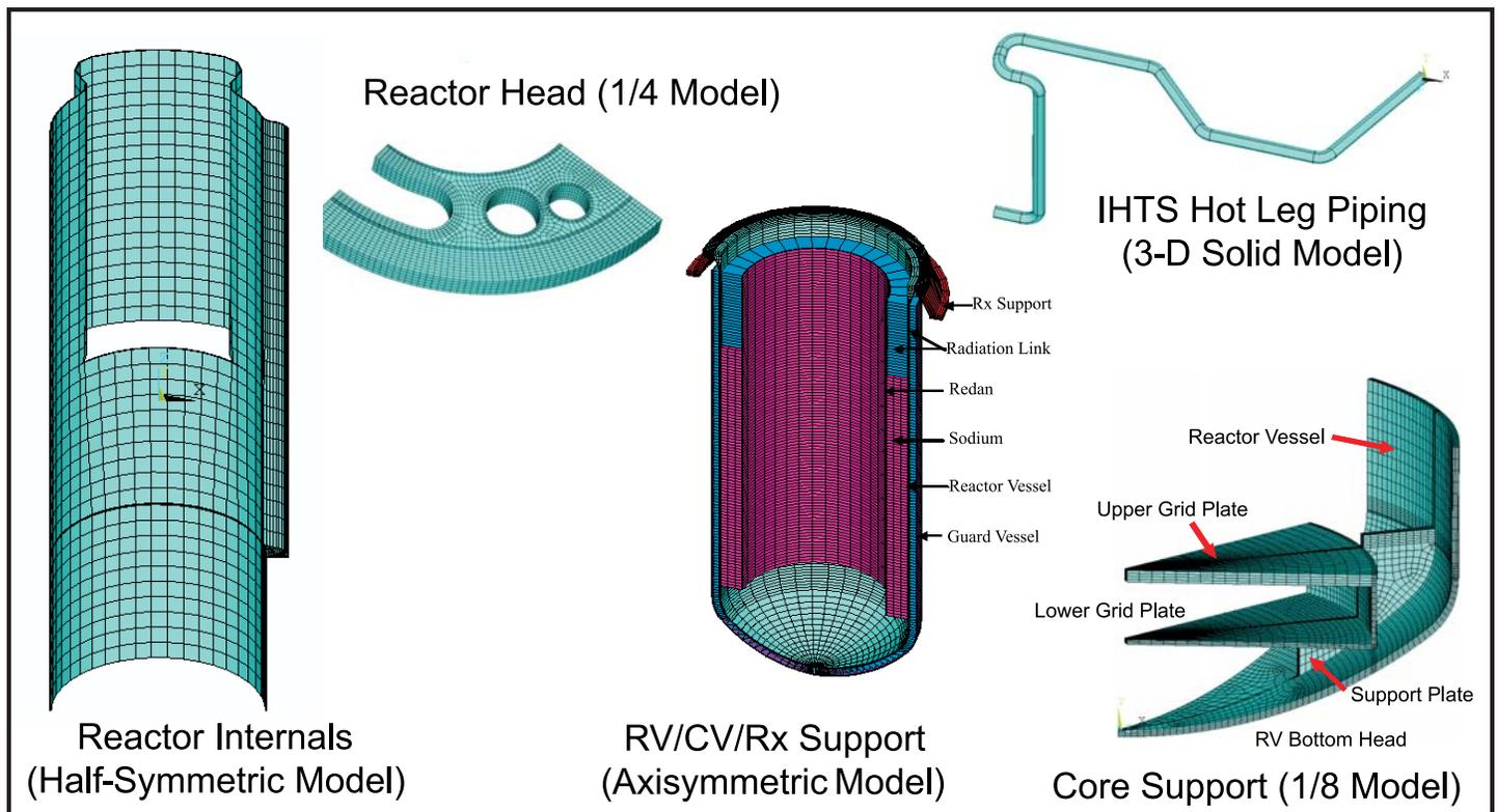
Figure 1. Finite element models for ABTR components for high-temperature design analysis.
