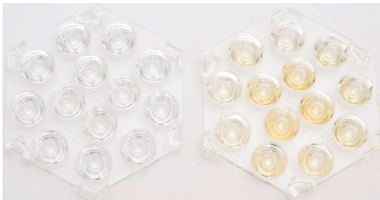
Figure 22. Secondary lenses taken from PAR38 LED lamps measured under accelerated testing showing the yellowing of the optic on the right after nearly 14,000 hours of testing due to excessive heat. The clear optic on the left shows the coloration after 2,000 hours of testing before the onset of yellowing. 9
