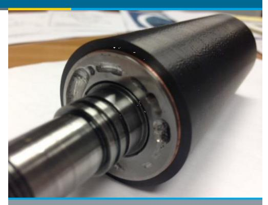
The electric machine being developed will incorporate a rotor with a composite sleeve and total harmonic distortion barrier to minimize rotor heating. Utilizing previously developed technology innovations will minimize project risk. *Photo courtesy of Calnetix Technologies*
