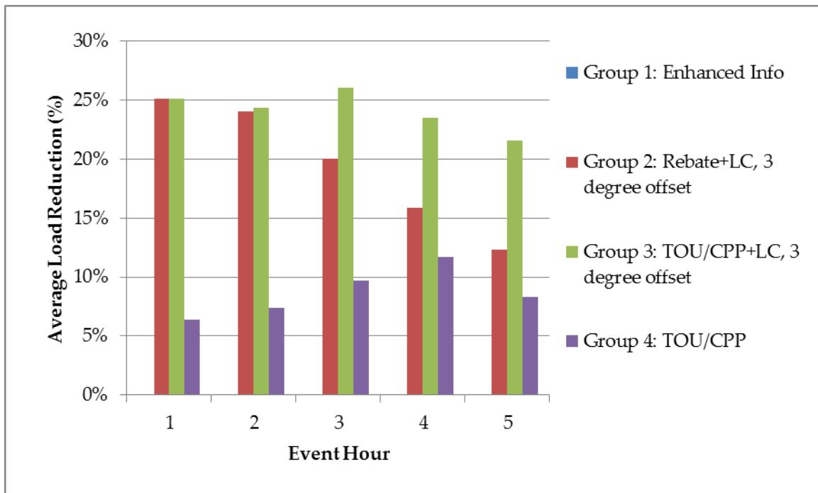
Results are based on data from 5-hour events with 3-degree offset; Group 1 did not demonstrate a discernible load impact.
