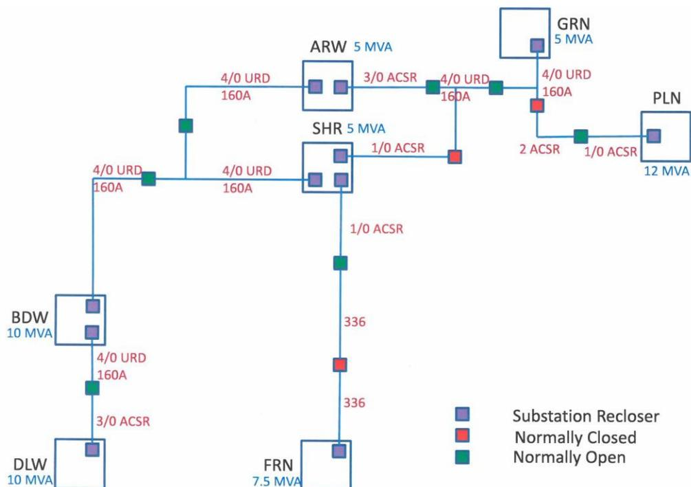
Figure 2. ACEC Substation Map with New Connectivity and Switch Settings
