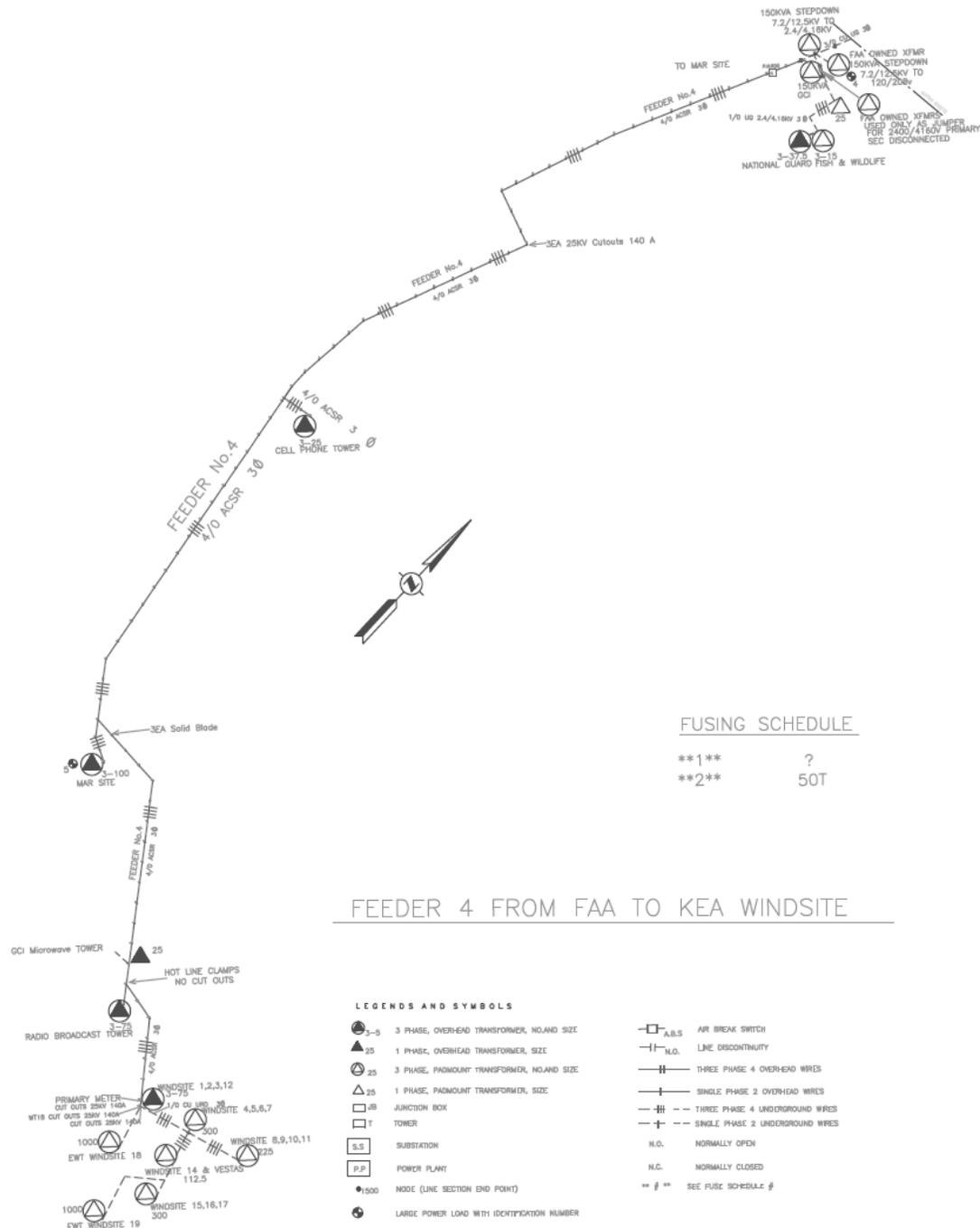
Figure 5. KEA Feeder 4 One-Line Diagram
