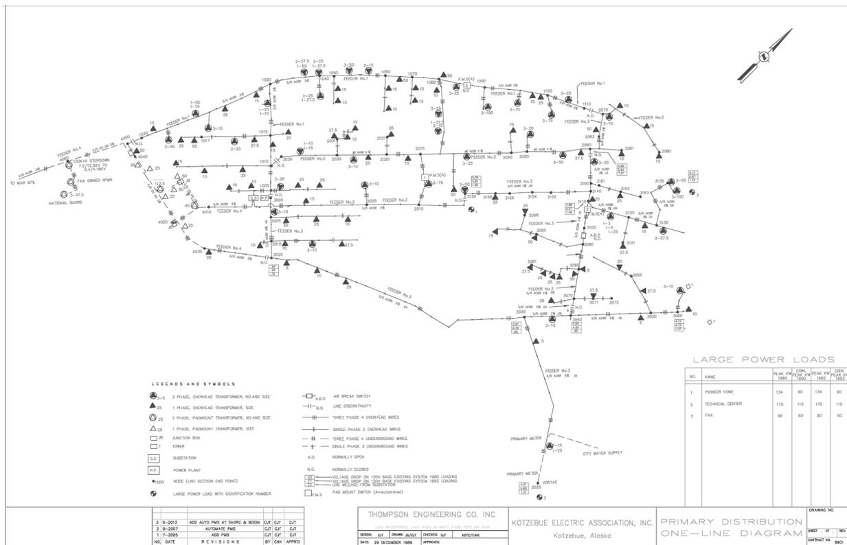
Figure 4. KEA Primary Distribution One-Line Diagram
