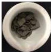
The lignin is a by-product of CTS milling process. It is separated from the product by taking advantage of its difference in polarity from the catalyst, and other biomass constituents. The lignin produced by this process (left) is chemically unmodified and is pale brown to gray in color.
