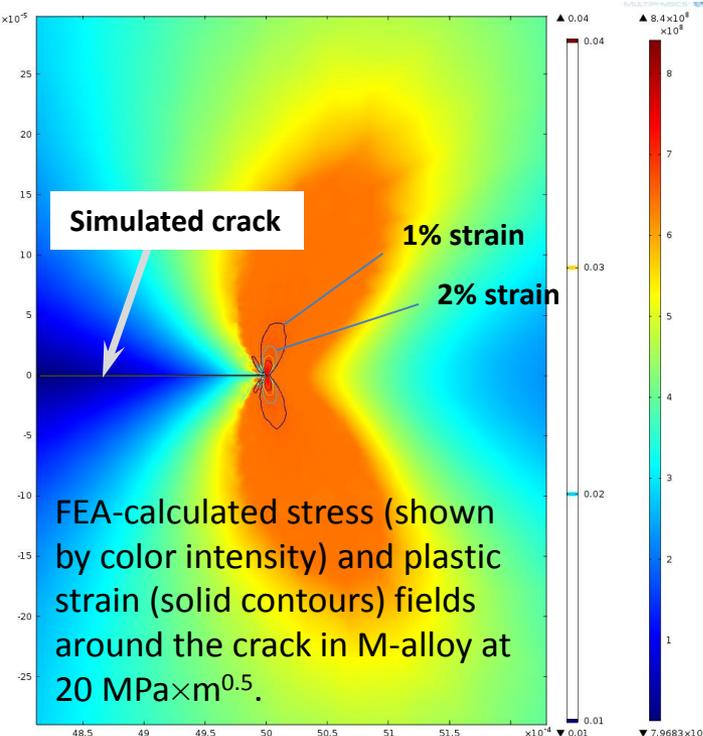
As was expected, stress concentration near the growing crack should lead to significant plastic strains in the crack-adjacent grains. The width of the area strained at  $\sim 2\%$  (EBSD-detectable strain level) was estimated to be  $\sim 20 \mu\text{m}$  micron on each crack side.
