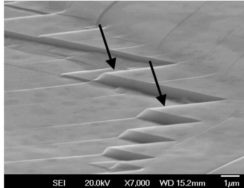
Non-irradiated steel demonstrates numerous, fine slip lines.
