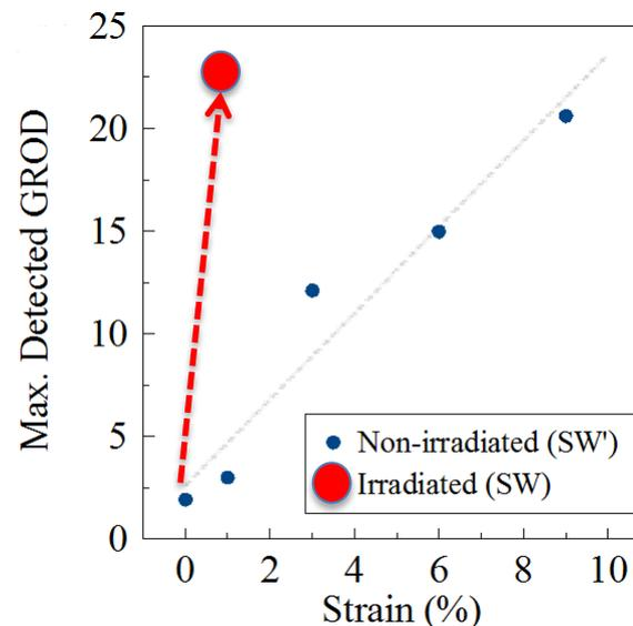
*Relationship between the maximum observed GROD value and strain level for non-irradiated and irradiated specimens.*
