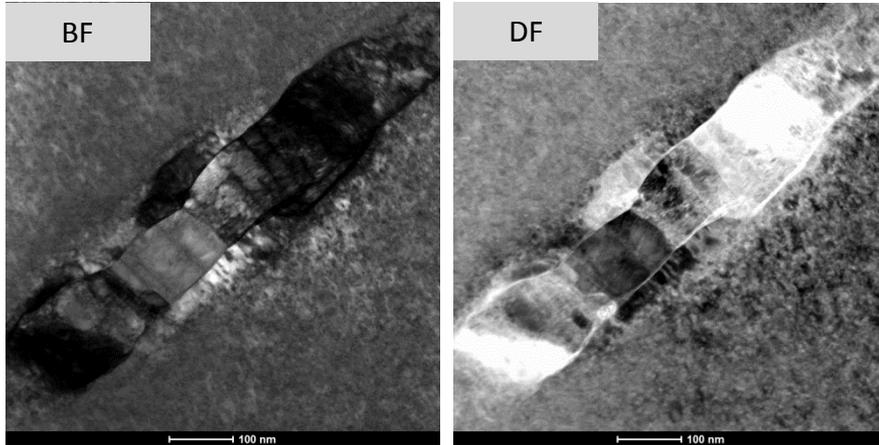
The “inclusions” were identified as areas with significant misorientation (several degrees) relative to the parent matrix and high dislocation density.
