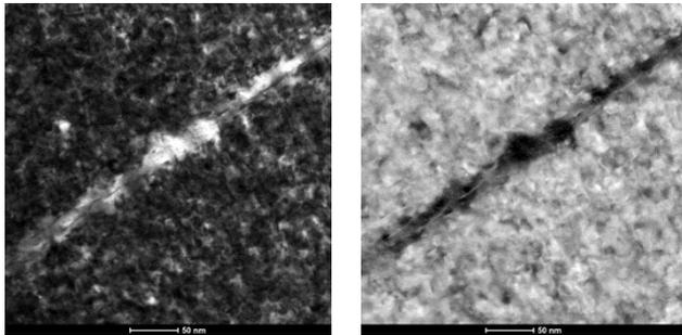
Internal structure of the dislocation channel. No twin was observed in this particular channel.
