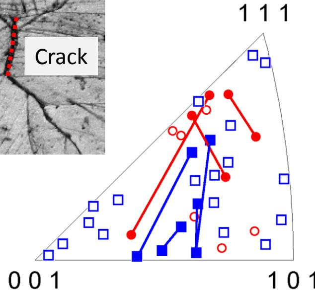
Typical EBSD maps (left) and IPF plot showing the orientation of crack-adjacent grains (closed symbols connected by line) and non-cracked (open symbols). The plot shows data for two scanned cracks (circles and squares, respectively).
