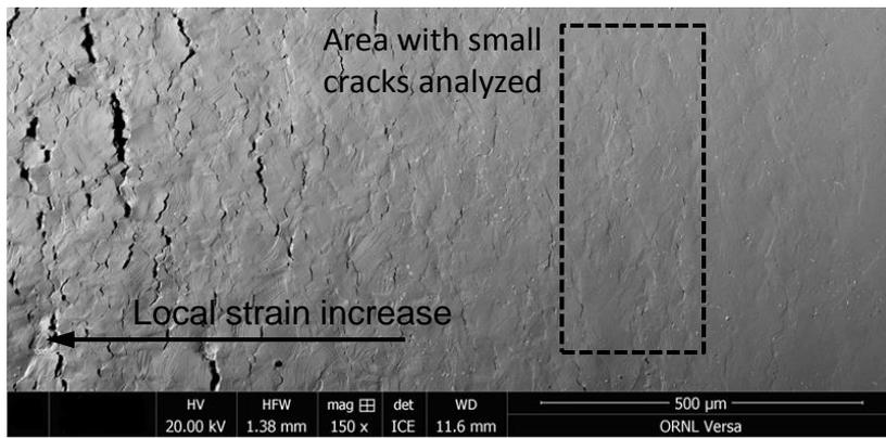
SEM-image showing a gradient in crack density.
