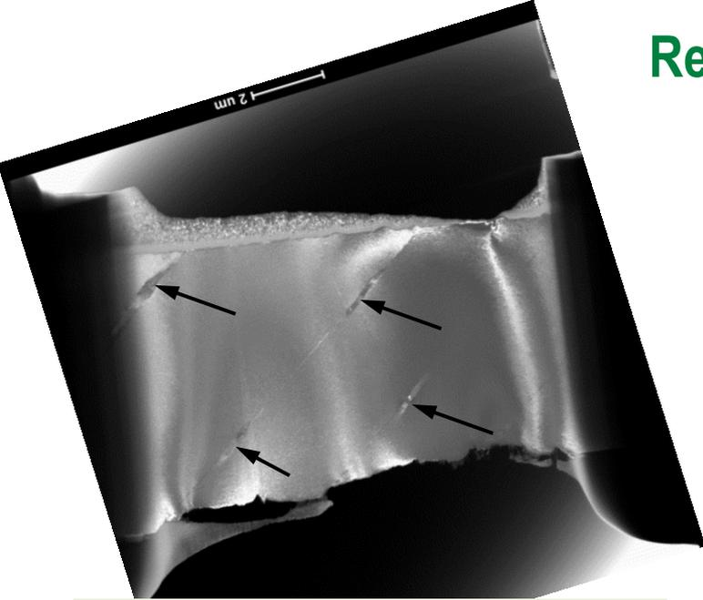
A FIB-liftout was performed at the crack-free location of 10.2 dpa 304L steel specimen. Local strains were small (<1-2%) and the sample was supposed to provide information on the near-surface oxidation processes and the local oxide structure near dislocation channels.
