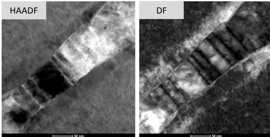
It appears, the radiation defect density inside the inclusion was lower compared to the matrix. Also, a shell with decreased defect density existed near the “inclusion”.
