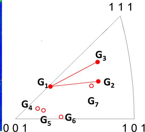
Cracks were analyzed in detail using SEM-EBSD to retrieve the orientation of crack-adjacent and neighboring grains. It gives an opportunity to investigate crack initiation in detail.
