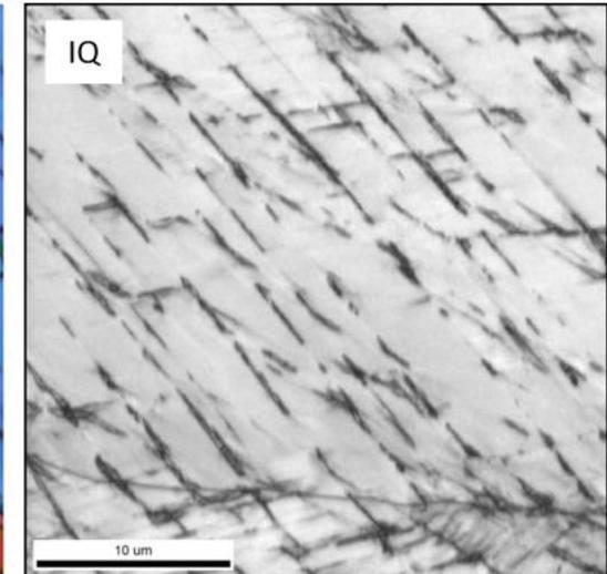
Fine EBSD-resolvable twins in 304L-specimen deformed in high-temperature water.
