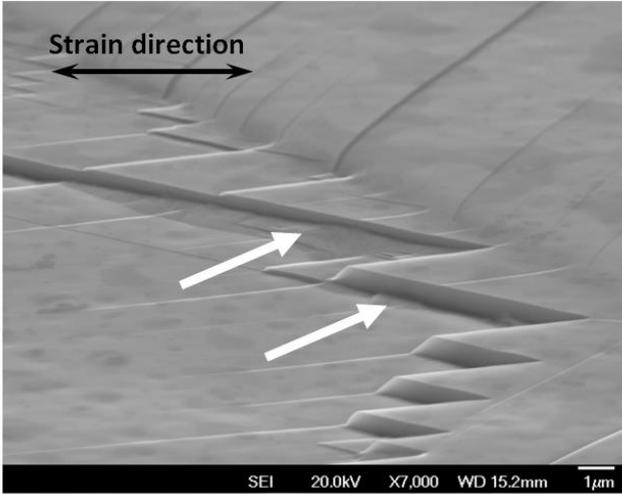
Specific martensitic transformation mechanism was observed at the irradiated specimen surface. Martensitic BCC-domains, identified and confirmed independently by EBSD and TEM, formed along the defect-free channels, if channel heights exceeded  $\sim 150$  nm.
