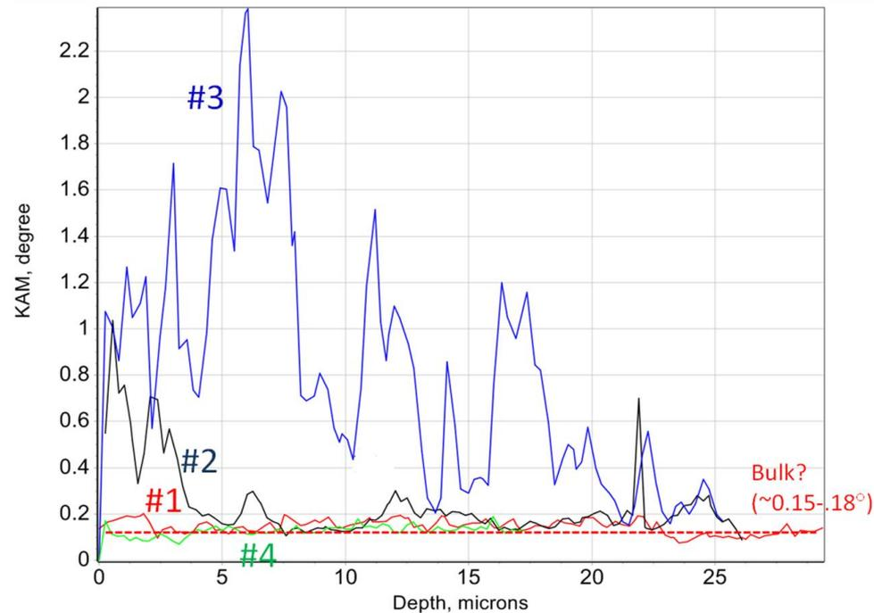
Kernel misorientation distribution at the crack edge. The diagrams show the detailed KAM profiles (#1-#4) taken at different locations.
