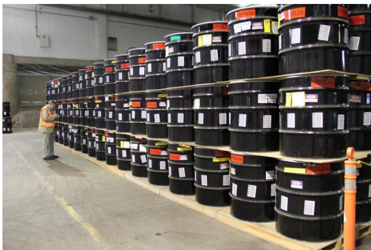
The white drums (above) are 55-gallon drums of waste, while the black drums (left) are 100-gallon product drums of waste, certified ready to ship to WIPP.
