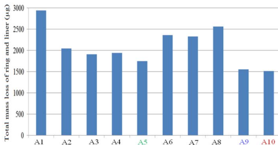
Figure 2. Wear mass loss of various antiwear additive combinations using the Plint ring and liner test at 100°C, 6 Hz, 240 N, 15 h test duration
