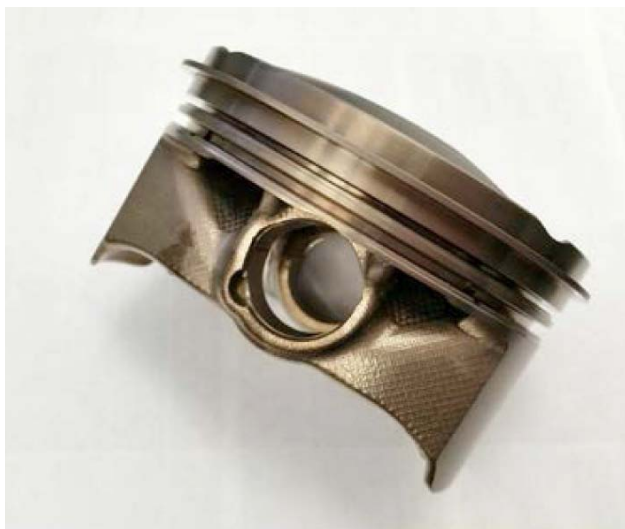
Figure 7. Piston-and-ring assembly coated with Argonne’s catalytically active non-ferrous coating.
