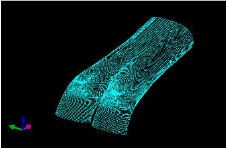
GridPro mesh for Intake Manifold of Sandia DISI engine taken from X-ray generated faceted surface
