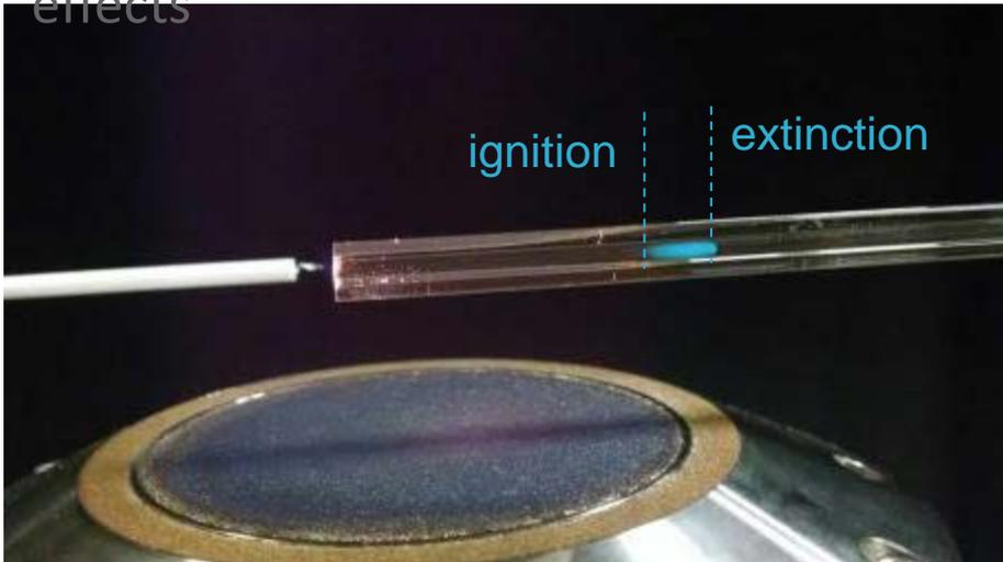
$\mu$ FIT prototype operating at LSU by Schoegl under the Co-Optima Fuel Properties team (propane shown)
