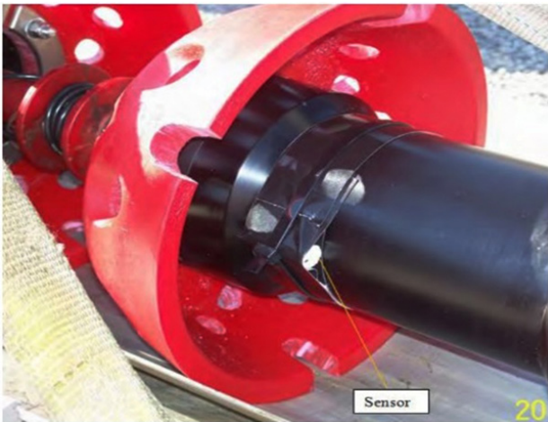
Figure 2. Location of sensor on magnetic flux leakage pig.
