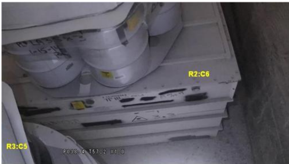
Figure 6-9: Undamaged Stretch Wrap at R2:C6
