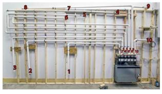
This mockup of the smalldiameter modular air distribution system that would be found in the chosen floor plan (upper left diagram on this page) contains the correct number and location of 90° bends, as well as the proper length of ductwork to fit the dimensions of the floor plan.
