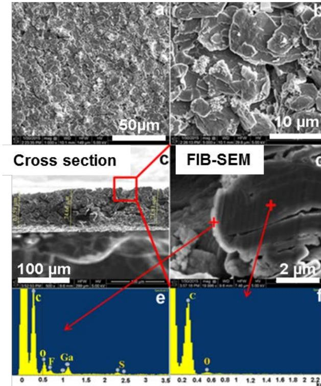
SEM/EDS of graphite electrode after cycled in graphite/sulfur battery.
