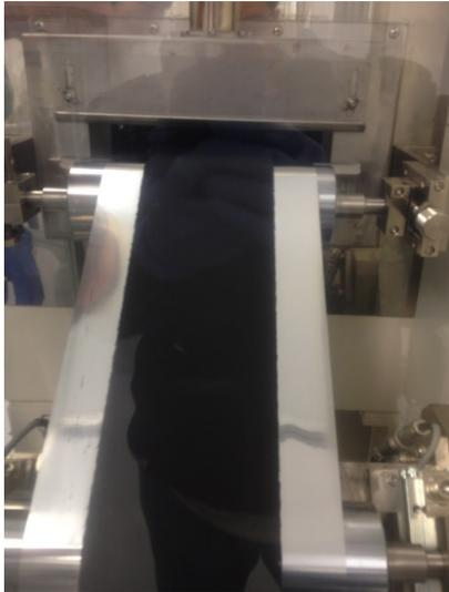
Double-side coated sulfur cathode
