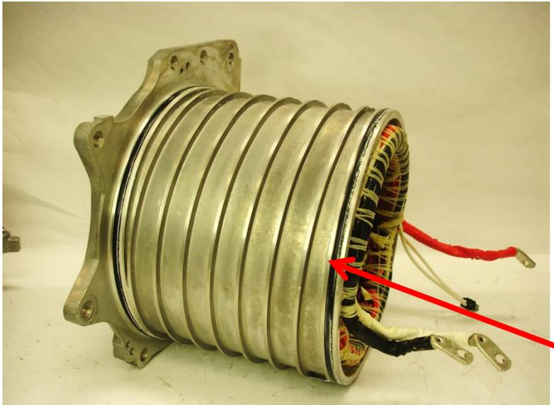
Spiral channel mates with outer housing for uniform cooling
