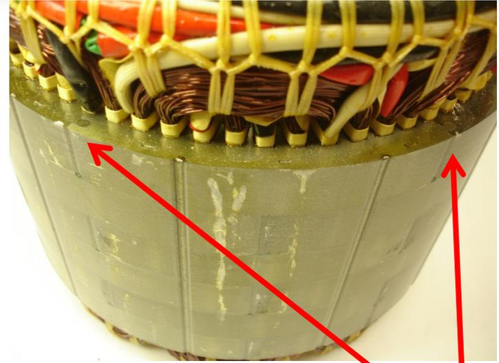
Stator laminations are made from separate pieces
