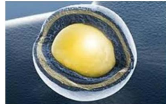
TRISO coated particle fuel
