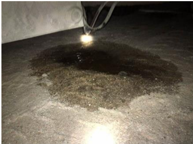
Figure 14: Hydraulic Fluid under Truck 74U006A
