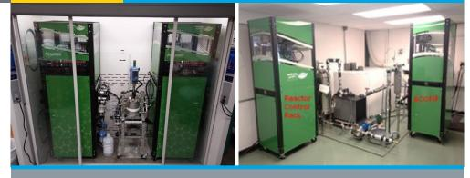
Academic researchers will develop basic control and automation technology using the laboratory scale Automatic Continuous Online Monitoring of Polymerization reactions/ Control Interface (ACOMP/CI) system (left). The technology will be validated using the pilot scale ACOMP/CI (right). *Photos courtesy of Tulane.*
