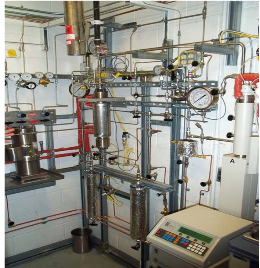
PNNL bench-scale, continuous-flow, fixed-bed, catalytic hydrotreater
