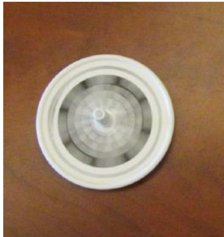
Flicker top showing stroboscopic effect Photo courtesy Aurora Ltg Design, Inc.
