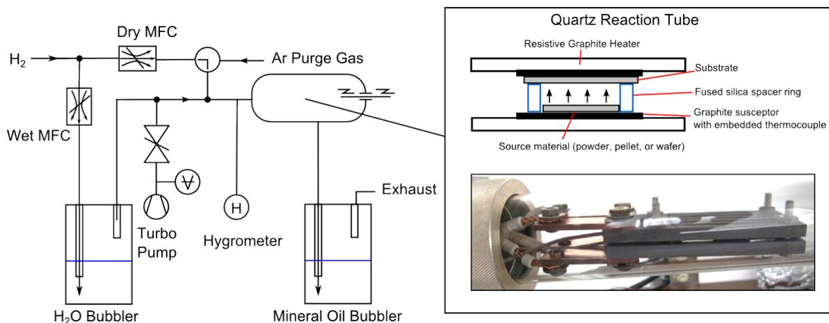
**Figure 1:** Schematic diagram of the custom CSVT reactor and reaction zone. Hydrogen gas containing water vapor reacts with GaAs to create volatile species in-situ. A temperature gradient between the
