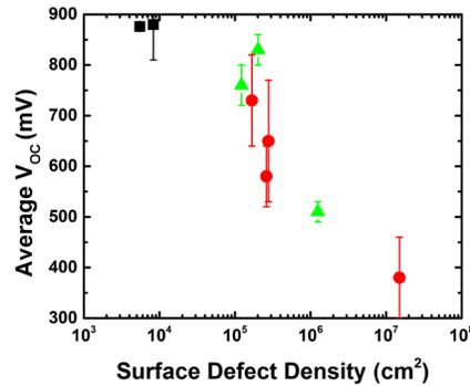
**Figure 14:** Average open-circuit voltage decreases with increasing absorber surface morphological defect density. Colors and marker shape indicate absorber films grown from different source pellets. Error bars show the standard deviation of the value for the 10 mesas fabricated from each *pn* junction. The data constitutes ~100 individual *pn* junction devices.
