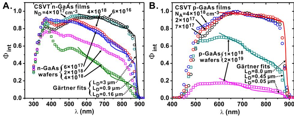
**Figure 5:**  $\Phi_{int}$  measurements obtained using PEC on  $n$ -GaAs (A) and  $p$ -GaAs samples (B). Experimental data is plotted as circles and calculated  $L_D$  fits from eqn. (5) are plotted as solid curves. The selected curves are representative of other electrodes obtained from the same samples and from other samples with similar free carrier concentrations.
