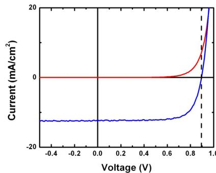
**Figure 10:** Light and dark IV curves for the 8.1% efficiency device from film 7.
