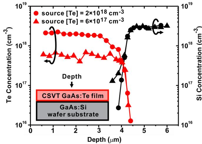
**Figure 2:** SIMS depth profiles of two *n*-GaAs films grown from differently-doped GaAs:Te sources on GaAs:Si substrates. The Te depth profiles are shown in red and Si in black. Circles denote the film was grown from a source containing  $[Te] = 2 \times 10^{18} \text{ cm}^{-3}$ , triangles denote the film was grown from a source with  $[Te] = 6 \times 10^{17} \text{ cm}^{-3}$ .
