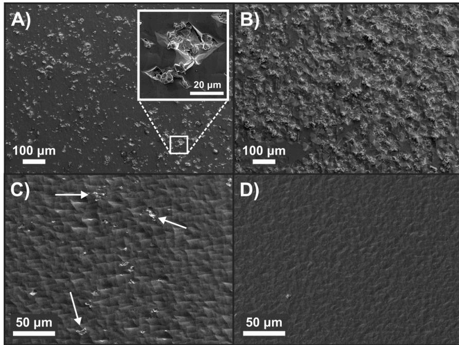
**Figure 22:** SEMs of **A)** varied composition sample  $[P] = 31\%$ , inset showing adventitious microstructure. **B)** varied composition sample  $[P] = 62\%$ , with more microstructures and surface texturing due to mismatch from the substrate. **C)** sample T1 ( $[P] = 30.2\%$ ), showing adventitious microstructures, some of which are indicated by white arrows, and a large degree of surface texturing. **D)** sample T10 ( $[P] = 27.7\%$ ), where microstructures are no longer observed.
