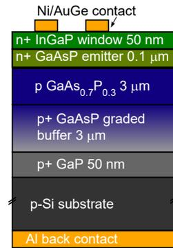
**Figure 35:** Target CSVT GaAsP on Si device.
