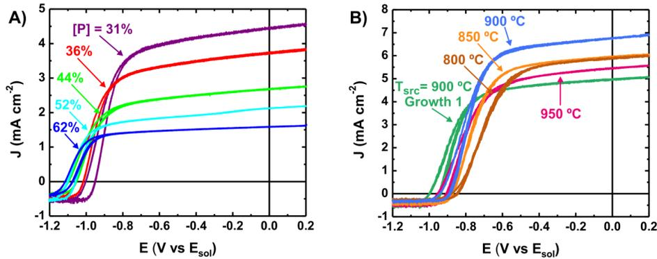
**Figure 24:** Representative JV curves. **A)** The decrease in  $J_{SC}$  across the composition series with increasing  $[P]$  is consistent with increasing  $E_g$  and the shift from direct to indirect  $E_g$ . **B)** The temperature series shows the best  $J-E$  characteristics for the samples grown at 900 °C; samples T3 and T5 have similar characteristics to T7 and therefore are omitted here. The compositional inhomogeneity of sample T1 (30.2%) appears to have reduced  $J_{SC}$ .
