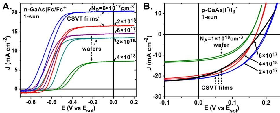
**Figure 4:** Photoelectrochemical  $J$ - $E$  curves of (A)  $n$ -GaAs and (B)  $p$ -GaAs CSVT films and control wafers. The curves are labeled with the corresponding sample's free carrier concentration in  $\text{cm}^{-3}$ . The selected curves are representative of other electrodes obtained from the same samples and from other samples with similar free carrier concentrations.
