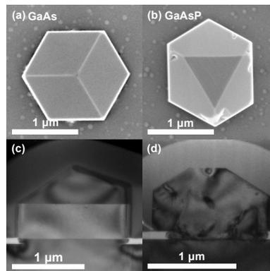
**Figure 31: A)** GaAs and **B)** GaAsP microstructure on GaAs (111) by selected-area epitaxy. **C)** and **D)** show cross-sectional TEM images prepared by FIB. The GaAs microstructures show twinning defects, while the GaAsP ones show a few interface dislocations due to the 1.3% lattice mismatch, but no twins.
