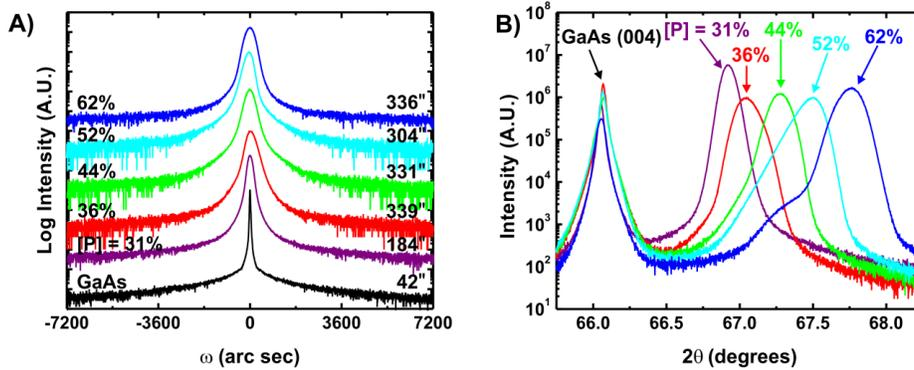
**Figure 19: A)** Rocking curve ( $\omega$ ) scans of each  $\text{GaAs}_{1-x}\text{P}_x$  (004) peak for the varied composition samples. FWHM values of all films are large compared to the GaAs substrate, a result of misfit dislocations. **B)**  $\theta/2\theta$  scans of the same samples, showing the shifting  $\text{GaAs}_{1-x}\text{P}_x$  (004) peak with increasing [P].
