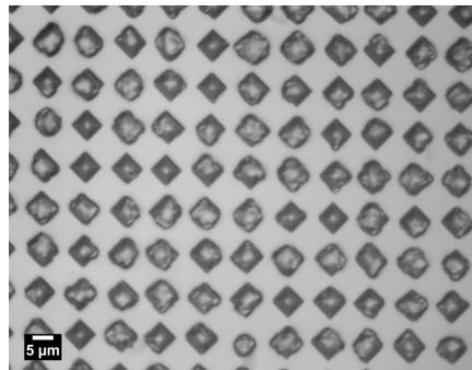
**Figure 33:** GaAs microstructures grown on Ge mesas, on a Si wafer. The Ge mesas were etched from ~50 nm films deposited by thermal evaporation on a (100) Si wafer, and subsequently treated by a cyclic thermal annealing process.
