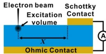
**Figure 6:** Schematic drawing of the EBIC experiment setup.
