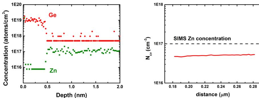
**Figure 12:** SIMS data from QSpec Technology (left) for device with both emitter and absorber grown by CSVT and capacitance-voltage profile (right) for a different device on the same film.
