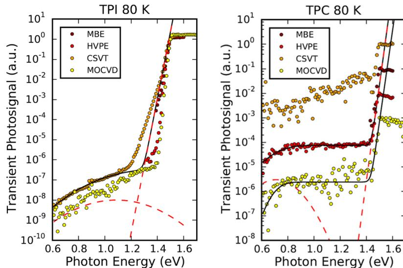
**Figure 17:** TPI and TPC spectra collected at 80 K for the four cells and corresponding fits. Some spectra were not fit since they did not fit the model of a single Gaussian distribution for the defect band.
