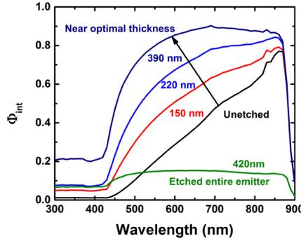
**Figure 11:**  $\Phi_{\text{int}}$  at various etch depths of the device from film 4 with both emitter and absorber grown by CSVT.
