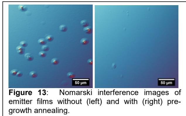
**Figure 13:** Nomarski interference images of emitter films without (left) and with (right) pre-growth annealing.
