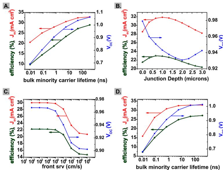
**Figure 8:** Simulations of  $p^+n$  devices using PC1D.
