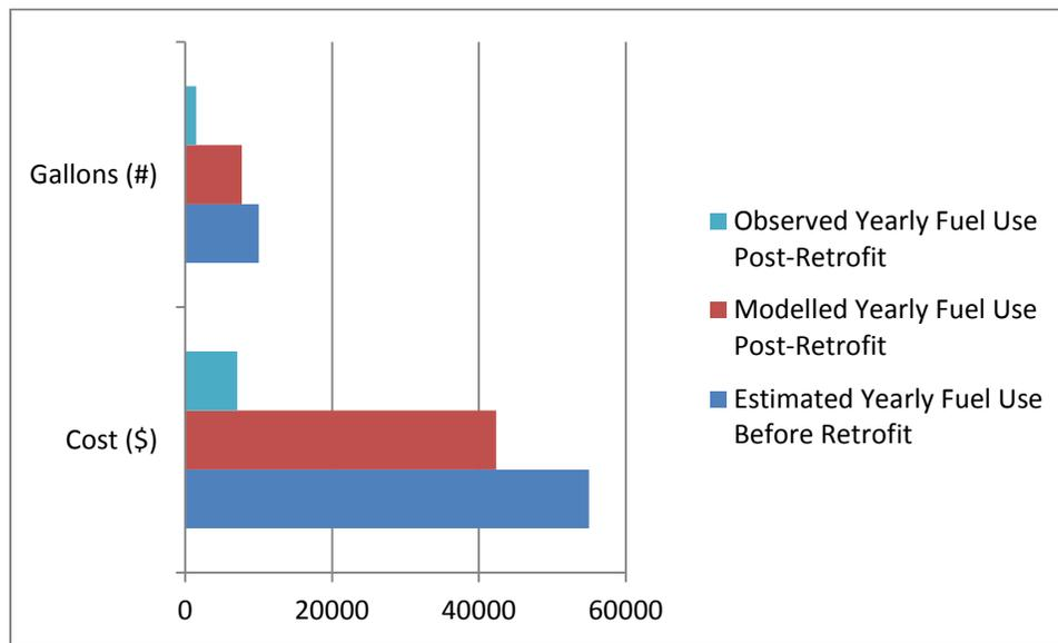
**Figure 7** This Graph shows the *estimated* fuel use pre project, the *modelled* fuel use post project and the *documented* fuel use post-project. We believe the actual post project fuel use lies somewhere closer to the modelled fuel use but still represents a reduction of 2300 gallons
