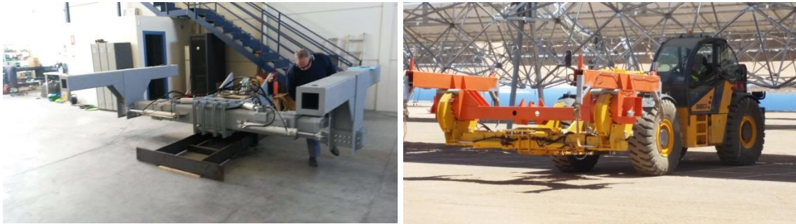
Figure 25: "Gripper" unit used for module installation
