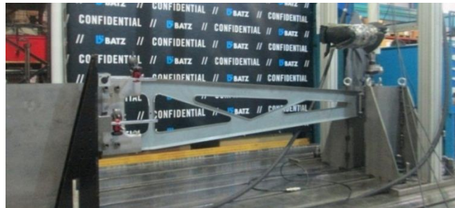
Figure 7: Batz stamped HCE support arm strength and stiffness test setup
