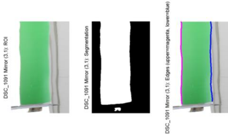
Figure 37: Distortion-corrected image of receiver reflection (top) and receiver image segmentation and edge detection (bottom)
