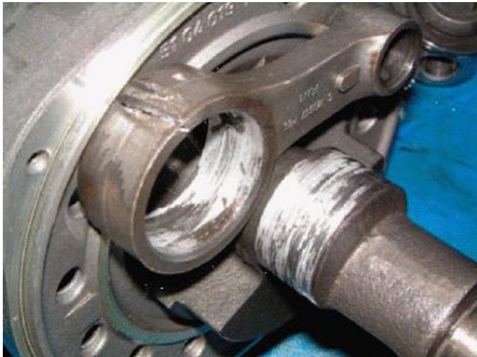
Broken connecting rod from liquid ingestion in compressor 4
