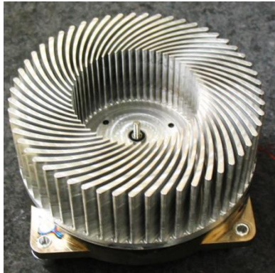
Sandia Rotating Heat Sink
