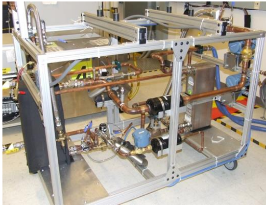
Calorimeter fabricated for compressor testing
