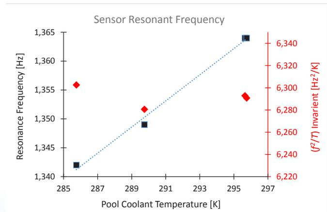
**Figure 4. Resonance frequency of the thermoacoustic sensor's standing-wave for different coolant temperatures demonstrating frequency is a function of temperature. The resonance frequencies corresponding to temperatures are plotted as black squares that spans  $\pm 1.7\%$ . The right-hand (red) axis has the same relative span, but the value of the  $f^2/T$  invariant [10], plotted as red diamonds, has a standard deviation of only  $\pm 0.12\%$ .**
