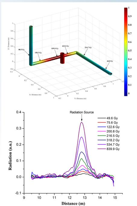
**Figure 3.** (a) Color-coded accumulated gamma radiation dosage by a Co-60 source after 120-minute radiation. (b) Distributed radiation dosage along the cable with various radiation times.
