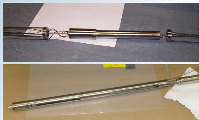
**Figure 1. “Fuel rod” thermoacoustic sensor. (Top) The thermoacoustic resonator is shown at the center of the photograph. (Bottom) The resonator and suspension springs are contained within a “slotted tube” that has the same outer diameter as the reactor’s fuel rods. The thermoacoustic sensor can be designed to meet the same geometrical constraints as most fuel rods.**
