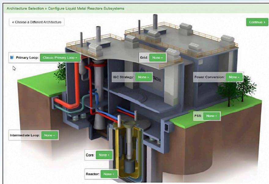
**Figure 2. A version of the web application developed by Modelon/Xogeny. The web platform allows for an advanced reactor concept configuration and parameter setting, which leads to a downloadable Excel and/or browser execution and simulation.**
