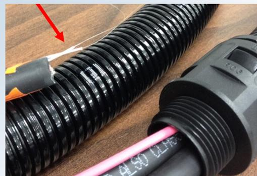
**Figure 1. A photograph of the electrical cable integrated with distributed fiber radiation and temperature sensors. The red arrow shows the inserted fiber protected by polymer tubing.**
