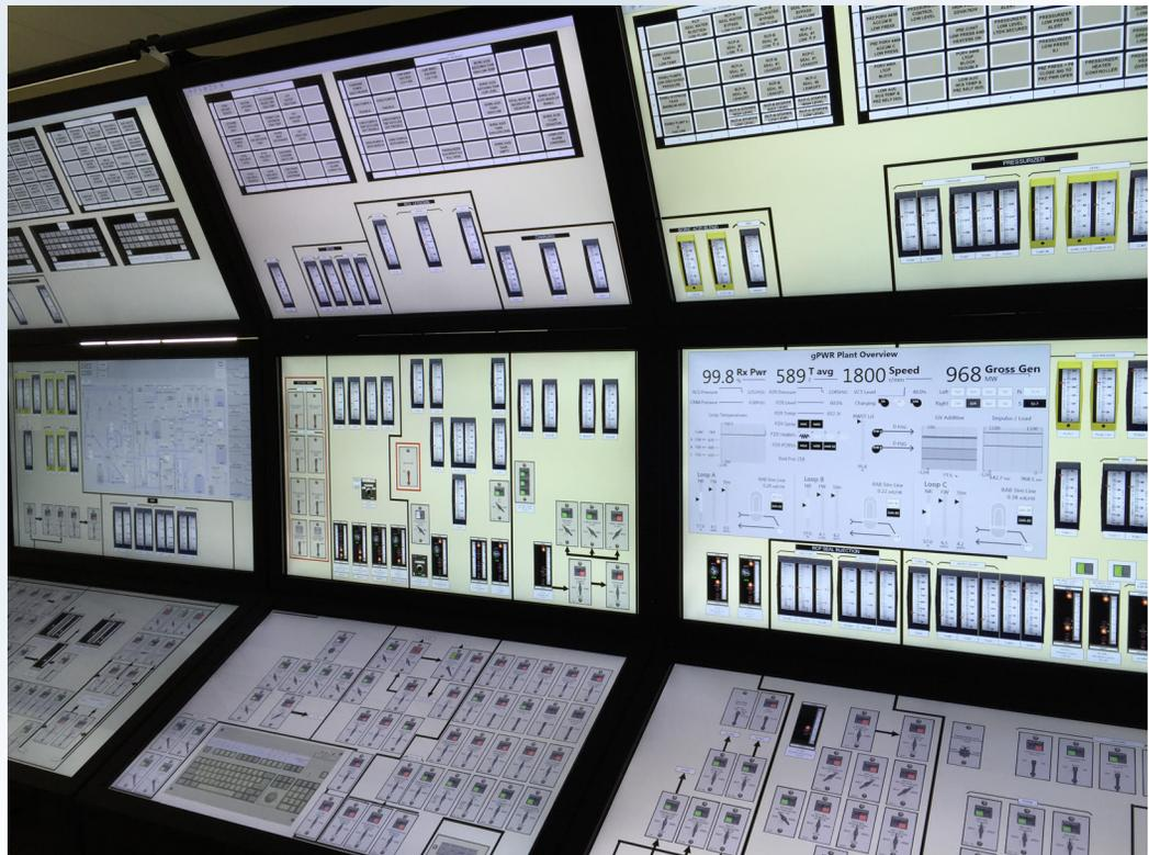
Figure 2. Computer Operator Support System (COSS) prototype embedded in the Human Systems Simulation Laboratory (HSSL).
