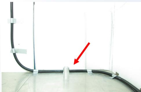
**Figure 2.** A photograph of the electrical cable mounted in the radiation chamber. The red arrow indicates the mock-up radiation source.
