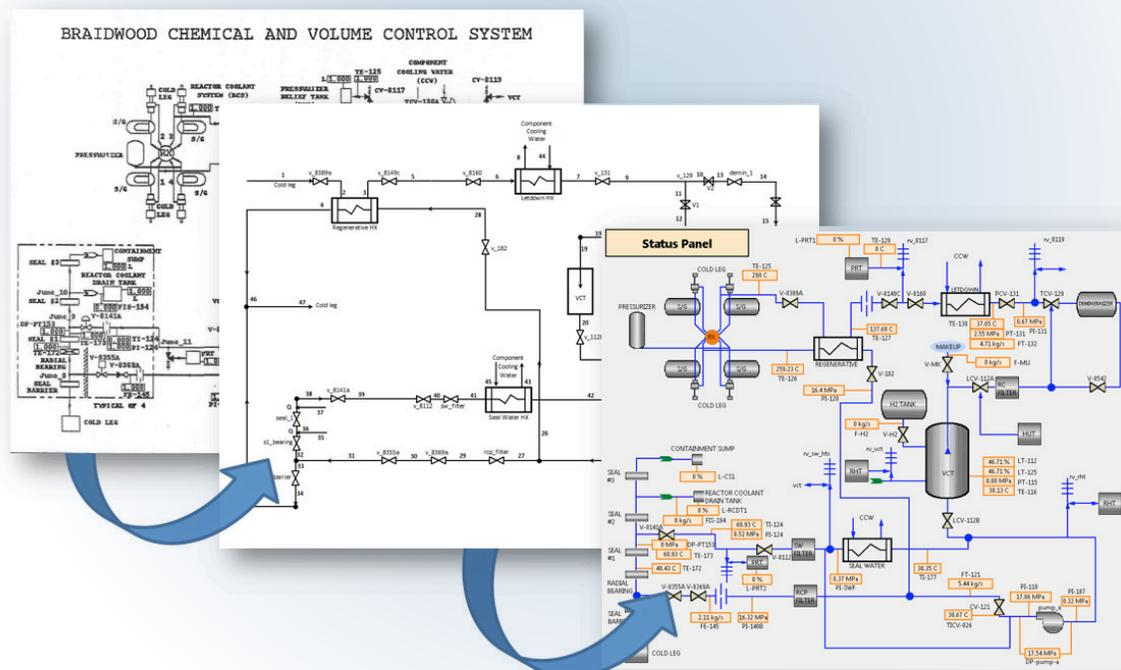
**Figure 1. CVCS physical system, the simulation model developed to describe it, and the piping and instrumentation diagram used in the validation of the fault diagnosis algorithms.**
