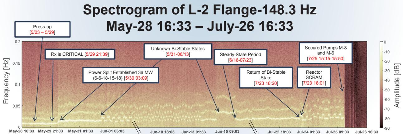
**Figure 5. Advanced Test Reactor vibroacoustic environment. Panoramic spectrogram view of a surrogate TAC signal produced by a five-vane pump, at 148.3 Hz, showing different ATR process states during the testing period from May 28 through July 26, 2015.**
