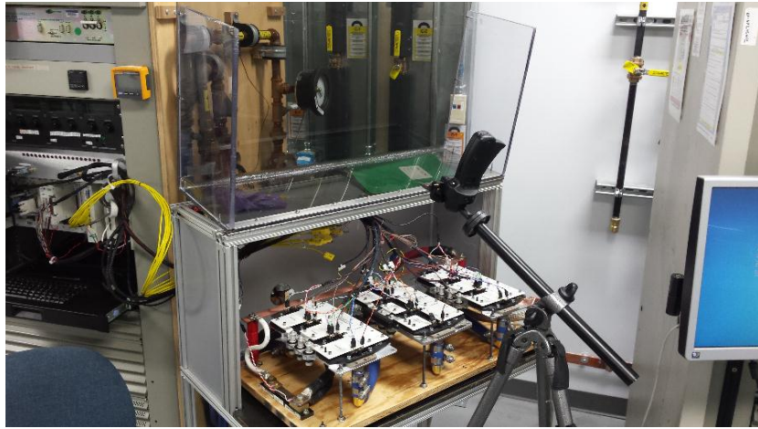
Figure 3-173: NGI Power Stages Being Prepared for Intermittent Operating Life Test General Motors
