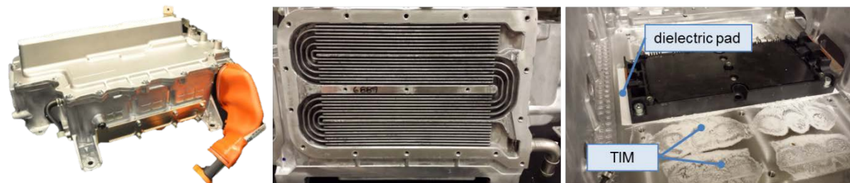
Figure 3-55: Pictures of the 2012 Nissan Leaf inverter. The middle image shows the cold plate cooling channels. Image on the right shows one power module mounted on the cold plate. The dielectric pad and TIM layers are shown (right).
