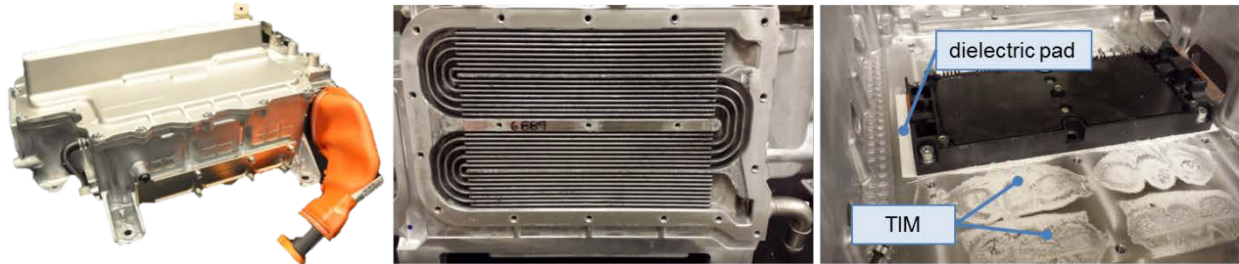
Figure 4-29: Pictures of the 2012 Nissan LEAF inverter. The middle image shows the cold plate cooling channels. Image on the right shows one power module mounted on the cold plate. The dielectric pad and TIM layers are shown (right). Photo Credit: Gilbert Moreno (NREL)
