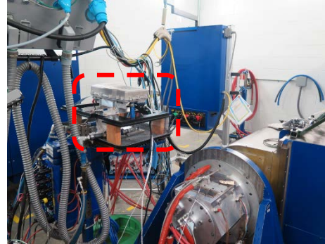
Figure 5: The Next Generation Inverter Prototype Under Active Load Test in GM's Dynamometer Laboratory
