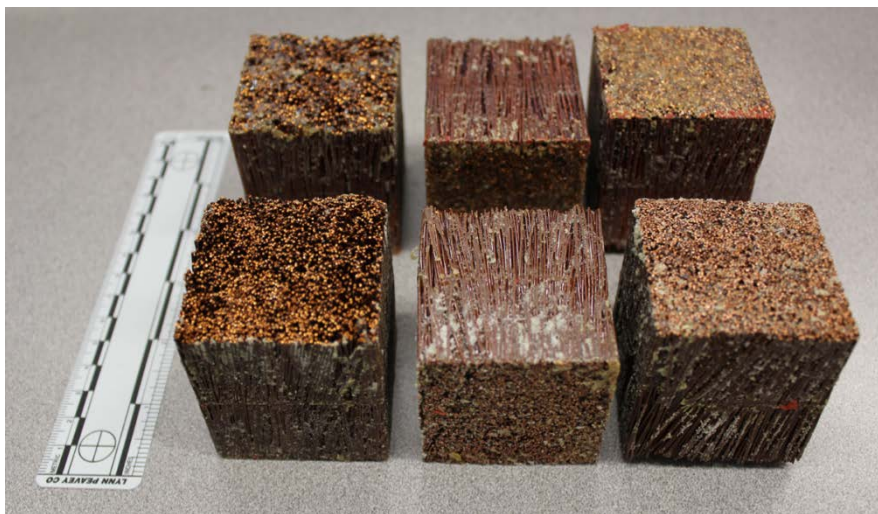
Figure 6-16: Custom copper-wound specimens were fabricated to facilitate the measurement of directional thermal diffusivity and thermal conductivity. Two copper wire diameters also were examined.
