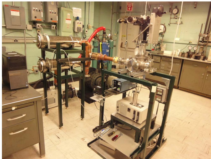
Figure 3-123: Photograph of the aerosol deposition system built at Argonne National Laboratory.
