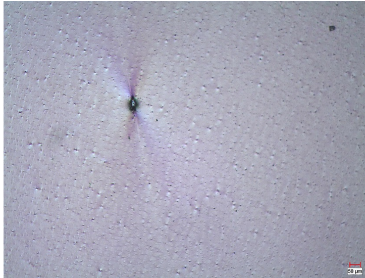
Figure 3-143: Polarized light images of a 5 \mu\text{m} PEI film surface showing subtle features (<10 \mu\text{m} ) and defects ( \sim 100 \mu\text{m} ).
