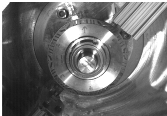
Figure 2-36: Image of 18 rotor laminates on test stand. Test rotor was spun to failure in vacuum.
