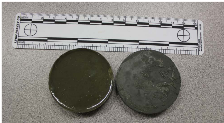
Figure 6-15: Examples of mineral-filled molding compounds fabricated at ORNL.
