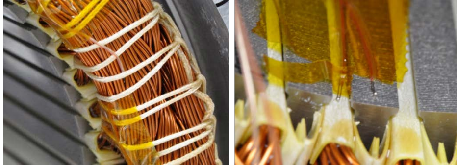
Figure 4-24: Pictures show the thermocouple placements on the end-windings (left) and stator surfaces (right).
