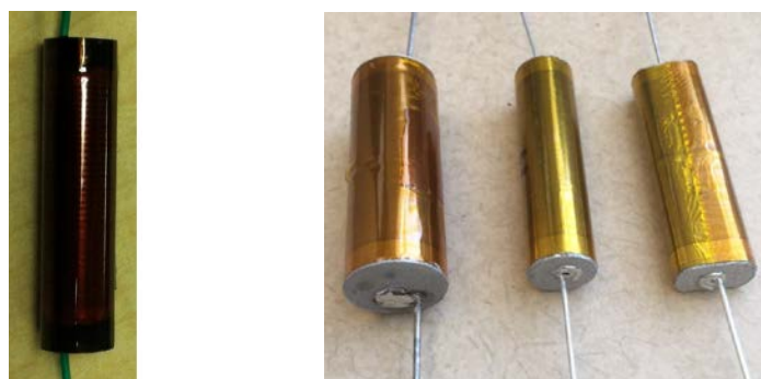
Figure 3-151: Image of an Epoxy potted capacitor made of 5 μm film from supplier A (left), and capacitor made of 5 μm film from supplier B (right).
