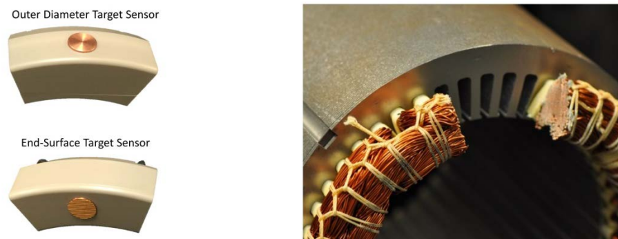
Figure 2-79: Assembled sensor packages for outer diameter surface measurement and end surface measurement (left), stator winding removed for sensor package (right)
