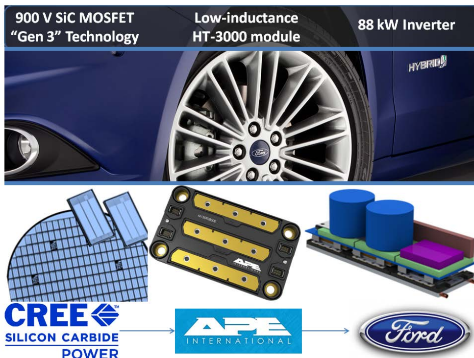
Figure 3-87: This work brought together a team which is leading the market in SiC power device production (Cree), SiC power module technology (Cree Fayetteville, formerly APEI), and HEV/EV platforms in the US market (Ford). Cree is the leading supplier of SiC and GaN components, including SiC power MOSFETs and diodes, and is also an automotive supplier of SiC diodes to HEV / EV platforms. Cree-Fayetteville is a leading producer of high-temperature and low-inductance modules, which take full advantage of SiC power devices. Cree-Fayetteville has also constructed automotive drive train prototype inverters in concert with other automotive OEMs on other efforts. Ford is the number one US producer of HEV / EV platforms, with a 13% market share in the US at the end of 2013.
