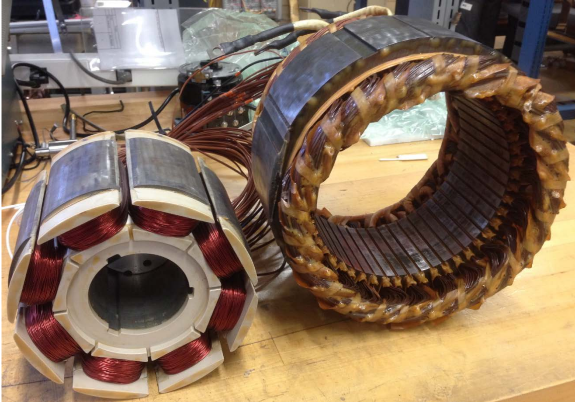
Figure 2-59: Wound and varnished WFSM prototype 1 rotor and stator.
