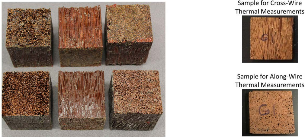
Figure 2-82: Winding sample blocks prepared by ORNL for thermal property measurements (left), cut samples prepared by ORNL and sent to NREL for directional thermal property measurements (right)
