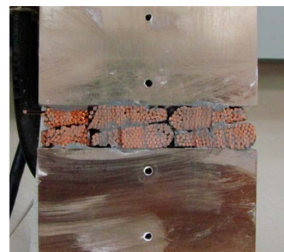
Figure 2-81: Images of sample slot-winding materials (left), sample slot winding under test for measuring cross-slot thermal conductivity (right)
