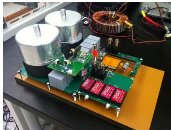
Figure 5-13: Photo of an experimental setup for evaluation of PBA SiC module electrical performance.
