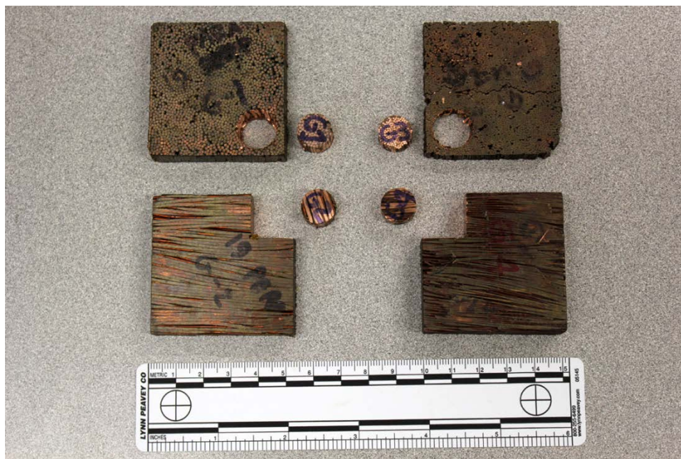
Figure 6-18: Core-drilled specimens were harvested from thin slabs of packed copper wire and used for thermal diffusivity measurements.
