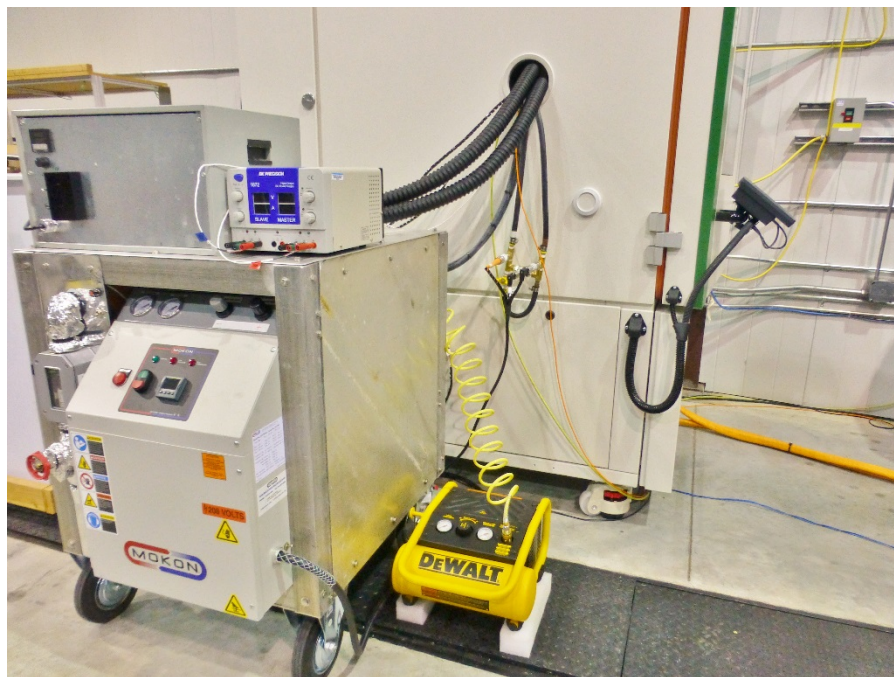
Figure 3-86: APEI designed and built housing containing a heater, pump, and air compressor to achieve a 105°C coolant loop temperature.
