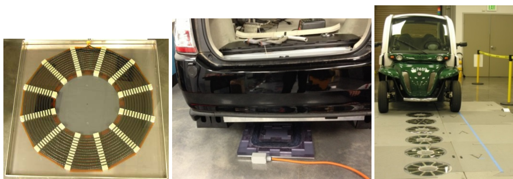
Figure 3-38: ORNL's previous work on add-on wireless chargers: coils (left), stationary wireless charging of a Prius PHEV (middle), in-motion wireless charging of a GEM EV (right).
