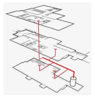
The standard domestic water heating packages offered at Stapleton include a conventional trunk-and-branch piping arrangement. In the sample home, the builder placed the water heater at one end of the basement, and hot water fixtures are spread out over the two floors above. The system has considerable piping length and excessive stored water volume between the domestic water heater (DWH) and the fixtures. An isometric diagram of the pipe to the most remote fixtures is shown at left.
