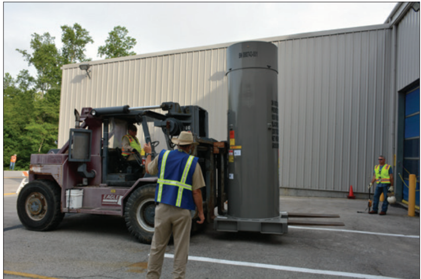
Workers move one of the newly designed remote-overpacks.
