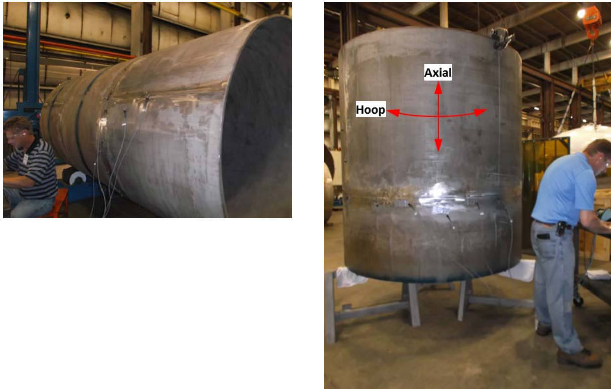
Figure 10: Measurement of strain gauges before (a) and after (b) cutting the container. The data acquisition system enabled four sensors to be monitored at a time, so that they were evaluated in groups. Sensors were measured using the same channel for the initial and final measurements.
