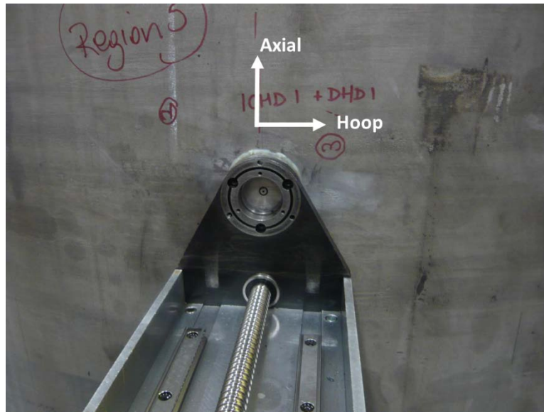
Figure 18: Positioning equipment used to perform DHD measurements of a base metal region (far from any weldments). The orientation of the axial and hoop stresses is indicated on the figure. In the center of the fixture, the hole and EDM overcore can be seen.
