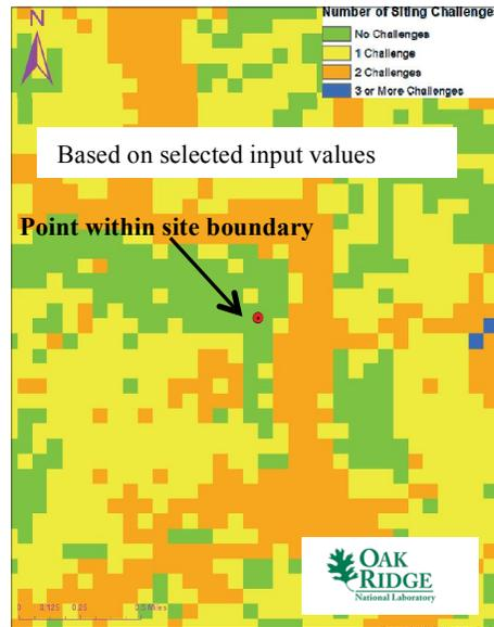
Fig. 2. Nominal, bounding SMR composite map detailing siting challenges for Chesapeake Power Station.
