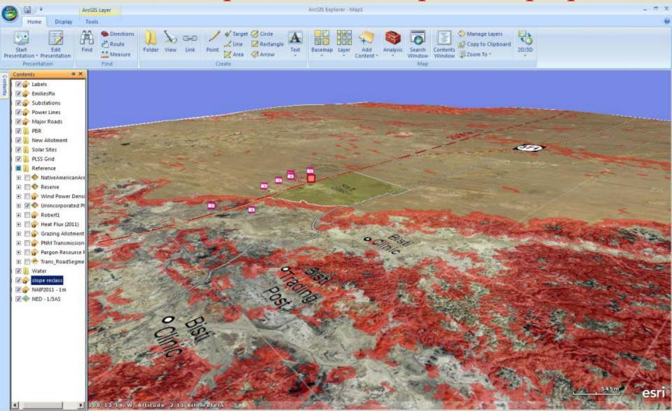
...to keystone Site #1: Bisti Substation, 230-kV line & Hwy 371 (data directory visible, slope layer turned on, >3% shown in red)
