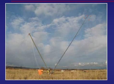
• Purchase or borrow and install two continuously recording, 60-meter tall anemometers stations equipped with modems to allow daily downloads of data – operate stations for one year.
