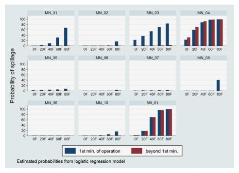
Probability of flue gas spillage for the 11 test sites. Sites MN-04 and WI-01 had improperly vented water heaters.
