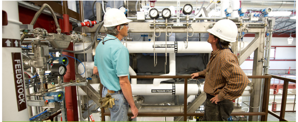
This continuous one-ton-per-day horizontal pretreatment reactor system has the capability for multiple configurations. Photo credit Dennis Schroeder / NREL
