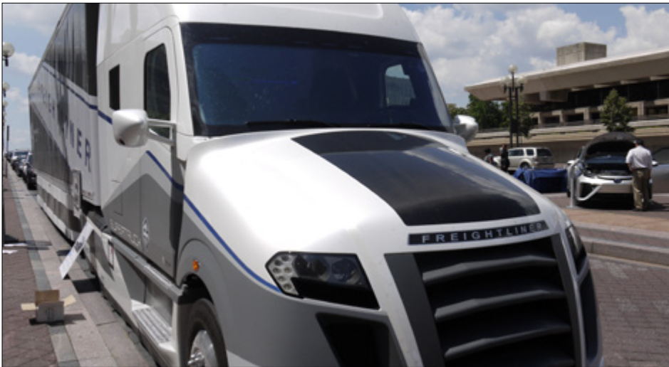
The Daimler Trucks North America SuperTruck gets 12.2 miles per gallon freight efficiency.
