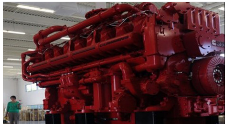
Cummins' Hedgehog is the world's largest high-speed diesel engine.
