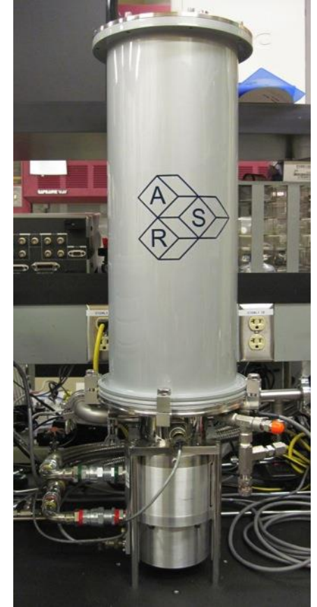
The entire system is enclosed in the vacuum shroud.
