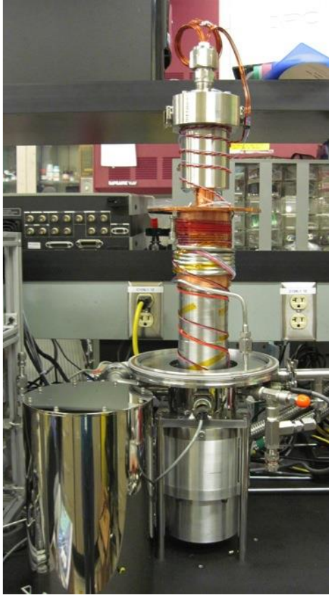
The pressure vessel mounts atop the cryo head.
