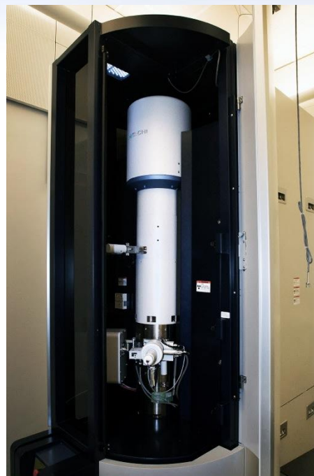
Hitachi HD2700C STEM Probe corrector
