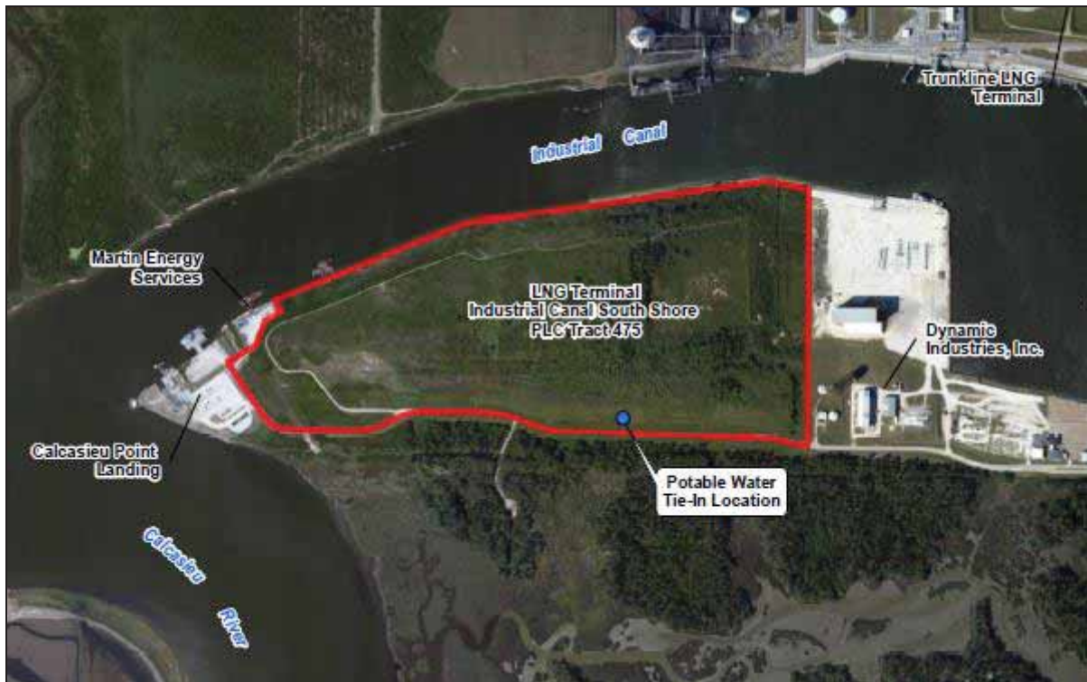
Figure 1.4.2-1 Tie-in to Existing Potable Water Line
