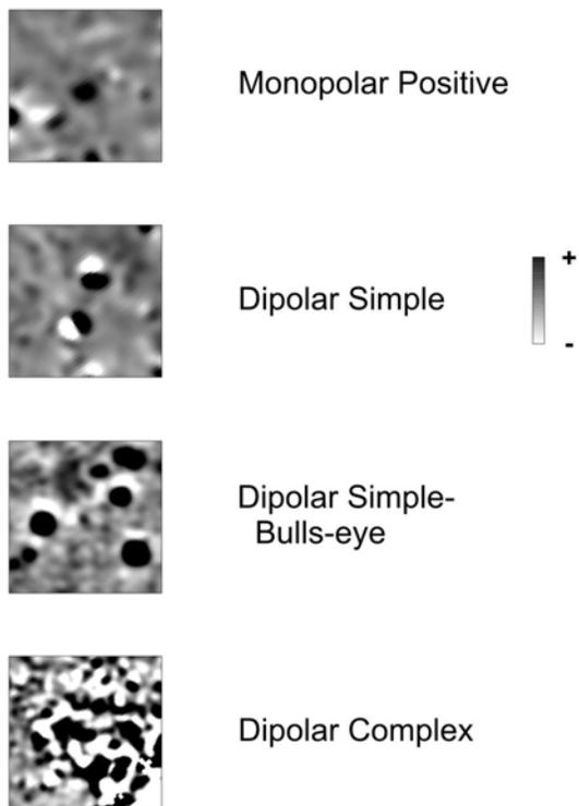
Figure 5.4. Magnetic gradient anomaly types.
