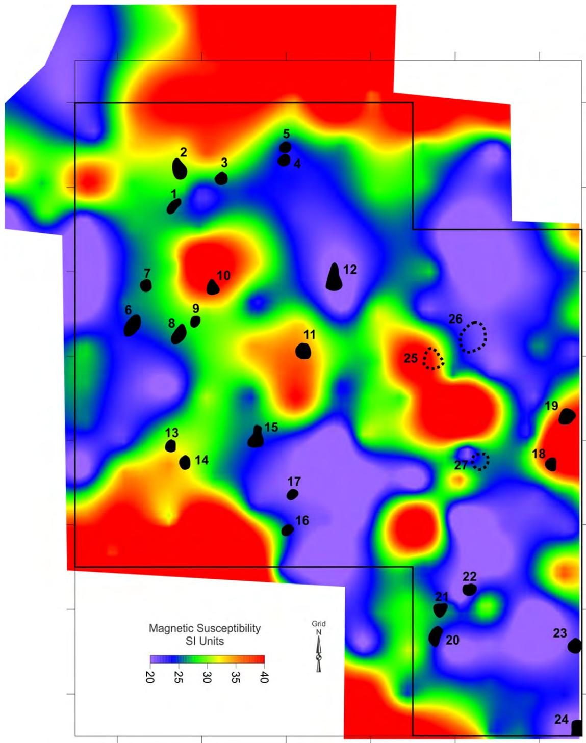
Figure 6.3. A map of magnetic anomalies of potential interest and the magnetic susceptibility survey results at 33Pk347.
