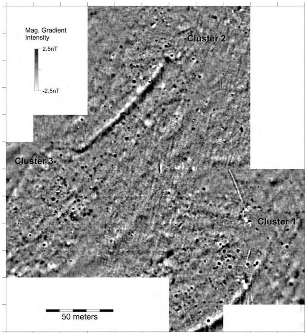
Figure 5.3. Example of magnetic gradient data from prehistoric Native American site, in this case the Brown's Bottom cluster of sites in Ross County, Ohio. Many of the small dark anomalies are archaeological features (see Pacheco et al. 2005, 2009a, 2009b for more on Brown's Bottom).
