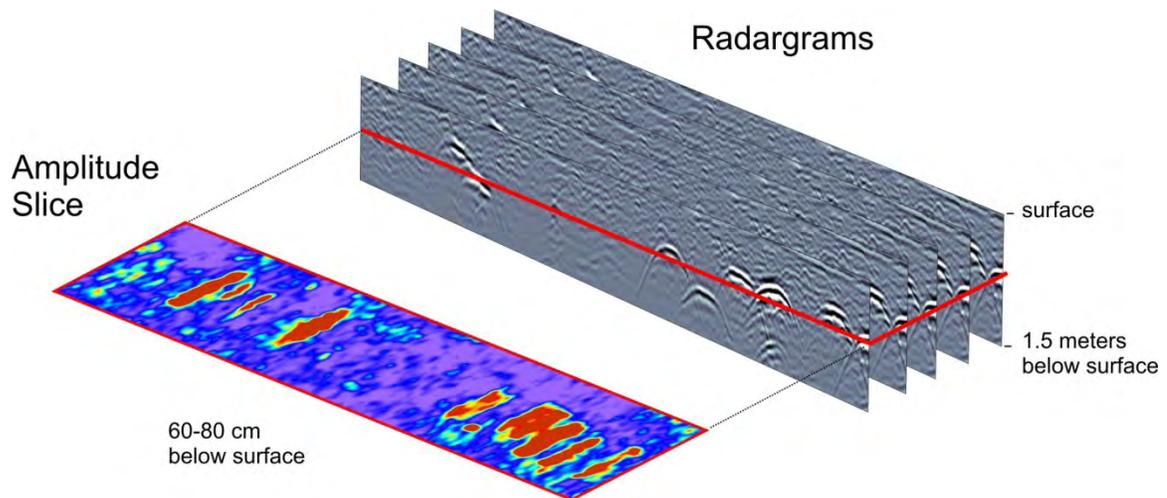
Figure 5.6. Creating amplitude slices from radargrams.
