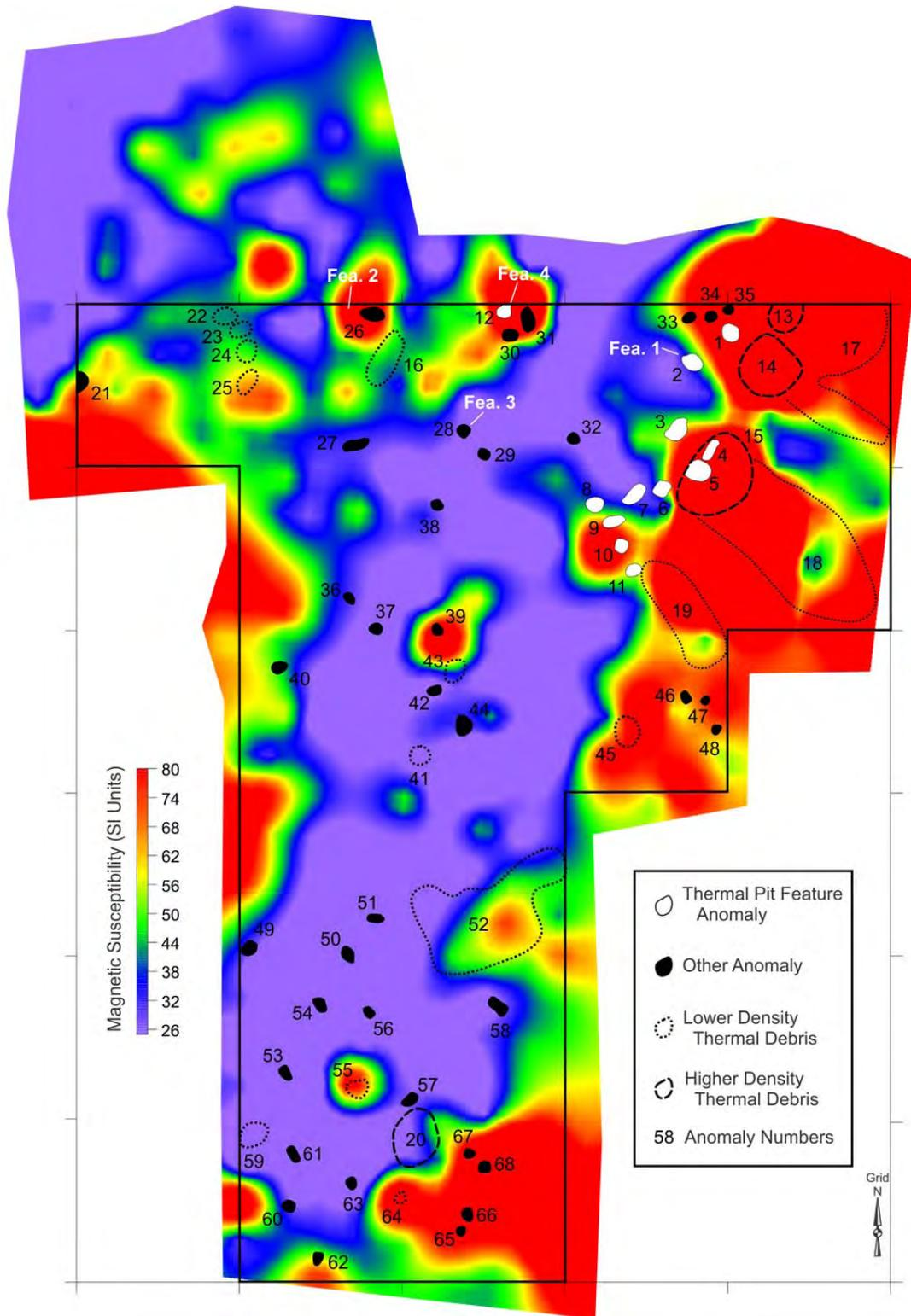
Figure 7.3. Magnetic gradient anomalies and magnetic susceptibility survey results at 33Pk348.
