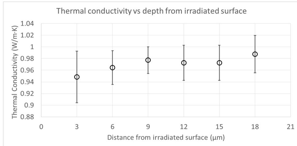
Thermal conductivity remains the same across the irradiated and non-irradiated region
