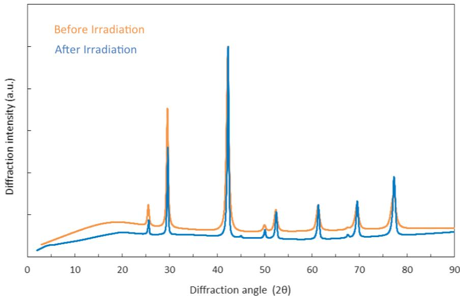
XRD pattern of the irradiated and non-irradiated *p*-type half-Heusler
