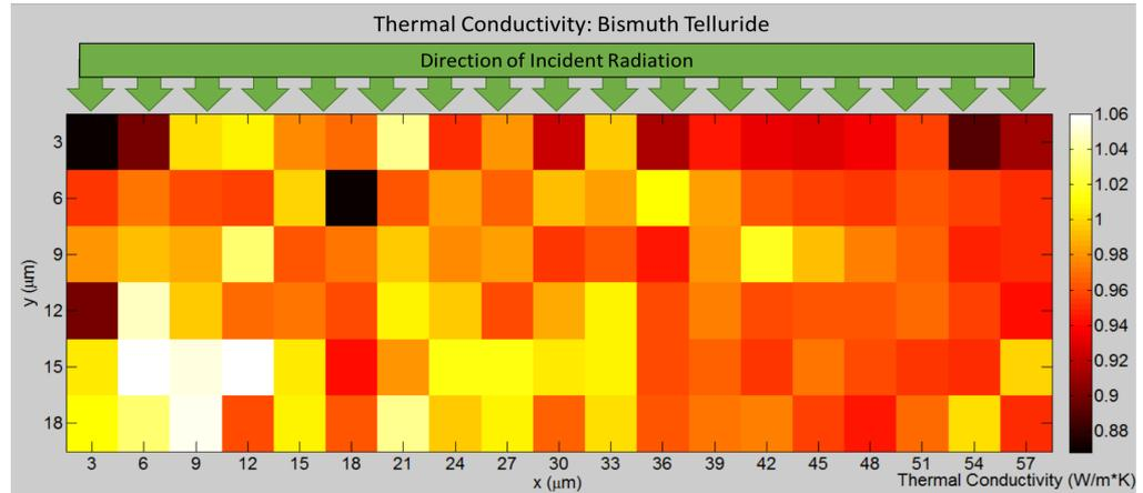
Thermal conductivity map of irradiated bismuth telluride cross section
