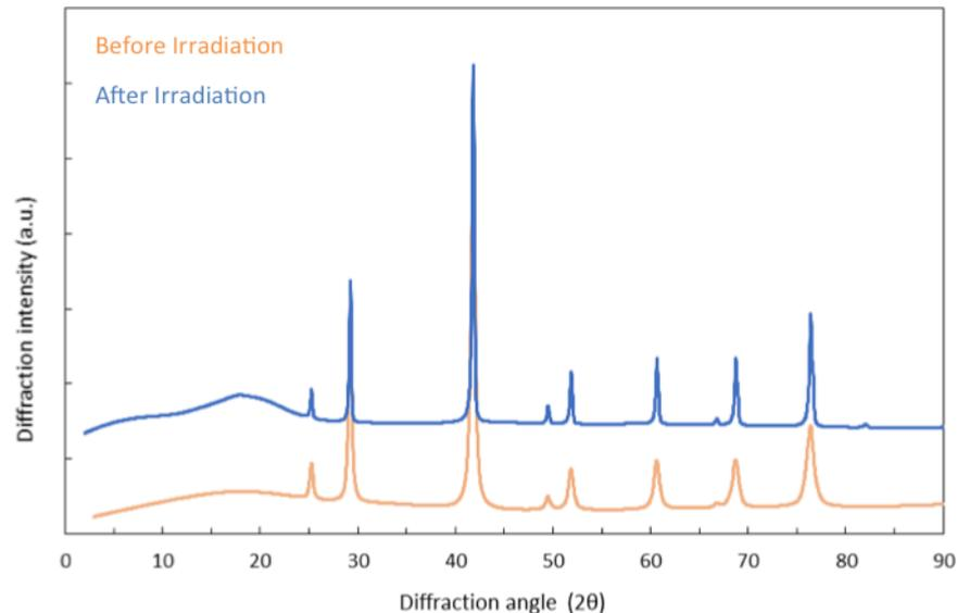
XRD pattern of the irradiated and non-irradiated *n*-type half-Heusler
