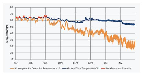
Crawl space condensation potential plot of a home without air conditioning
