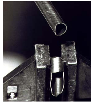
Austenitic Stainless Steel Following Irradiation in EBR II Fast Reactor
