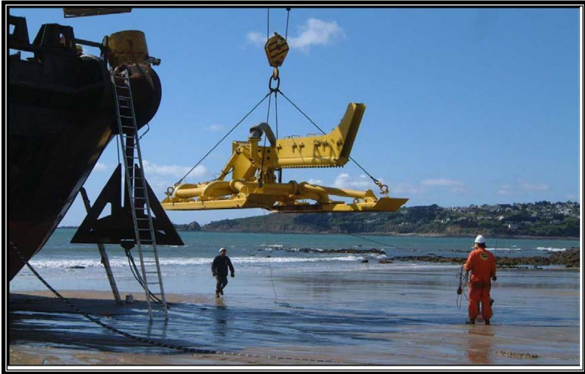
FIGURE 2-12 EXAMPLE OF WATER JET TRENCHING (JET PLOW) DEVICE
