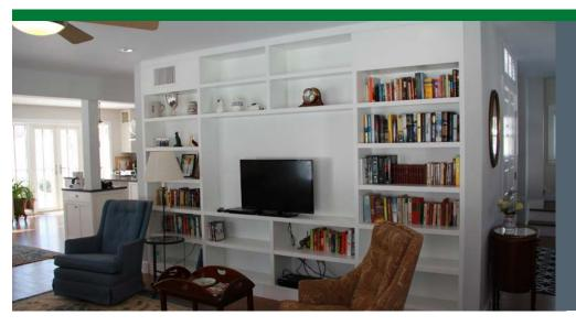
High-efficiency ducted heat pumps are installed in central locations on the first and second floors to provide heating and cooling through very short duct runs that are located within the home's conditioned space. A first-floor supply register is visible here above the book case. The second-floor ducts are located in a ceiling cavity between the drywall ceiling and a plywood attic floor.
