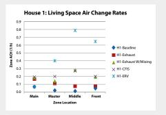
The CFIS and exhaust with central system mixing showed the best uniformity of zone air change rates.
