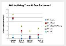
One-third of the outside air for the exhaust ventilation system in House 1 came from the attic.
