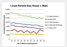
Exhaust ventilation showed the highest particle counts; CFIS showed the lowest particle counts because of improved air filtration.
