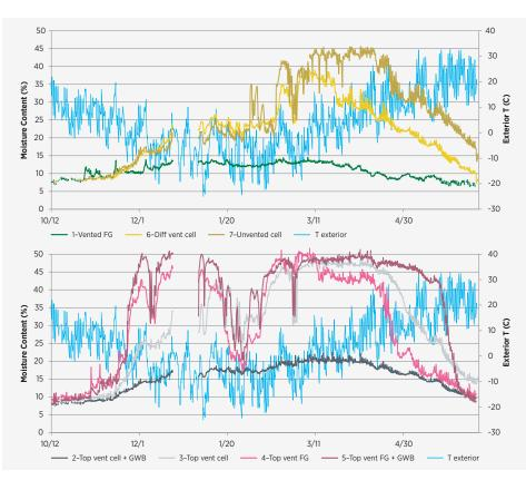
Rafter-framing top moisture contents in experimental roofs
